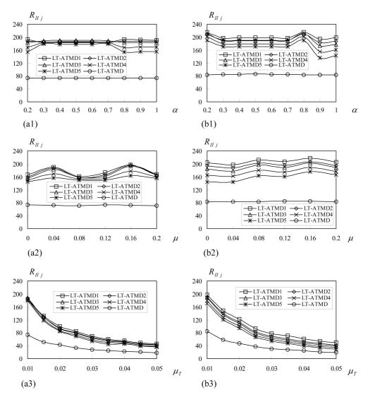
Fig. 6 Variation of the  $R_{IIj}$  value of the LT-AMTMD (including the LT-ATMD) with respect to the  $\alpha$  value with n=5 and  $\mu_T=0.01$  and  $\mu=0.03$  [(a1): r=-0.4; (b1): r=-0.8] and the  $\mu$  value with n=5 and  $u_T=0.01$  and  $\alpha=0.3$  [(a2): r=-0.4; (b2): r=-0.8] and the  $u_T$  value with n=5 and  $\alpha=0.3$  and  $\mu=0.03$  [(a3): r=-0.4; (b3): r=-0.8]
