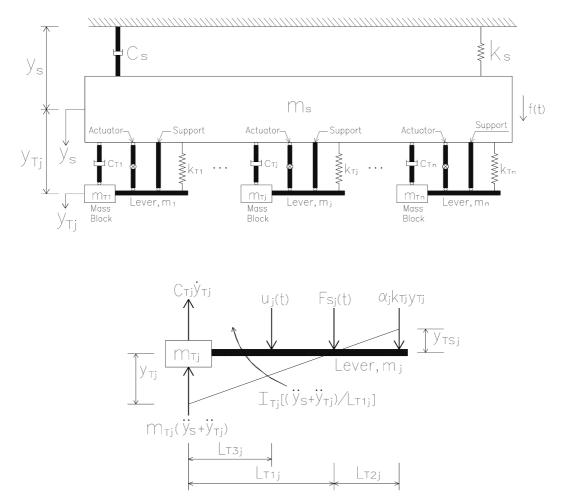
Fig. 1 Schematic diagram of the LT-AMTMD structure system
