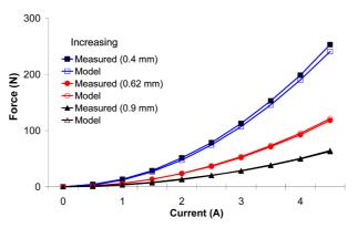
Fig. 5 Measured and calculated forces versus current for several air gaps
