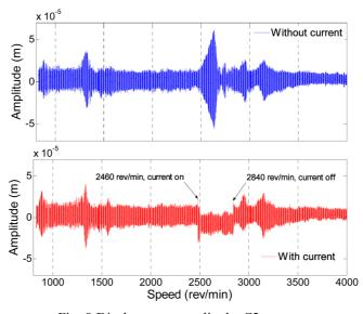
Fig. 8 Displacement amplitude, C2, run-up
