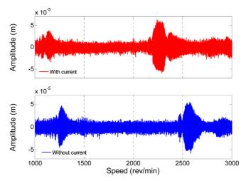
Fig. 7 Displacement amplitude, C2, 800 to 4000 rev/min in 30 sec
