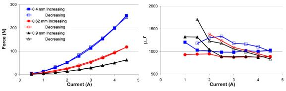
Fig. 4 Measured forces and relative permeability versus current for several air gaps
