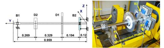
Fig. 1 Experimental test rig
