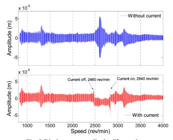
Fig. 9 Displacement amplitude, C2, run-down
