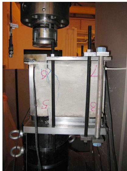
Fig. 6 Experimental setup and failure mode of direct-shear test
