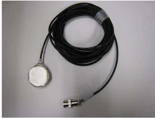
Fig. 1 Cement-based piezoelectric sensor
