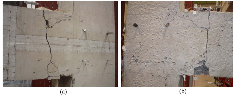
Fig. 9 Crack pattern of specimens after being subjected to cycles up to 72 mm (2.83 in): (a) front face of JBC-2 and (b) rear face of JBC-2
