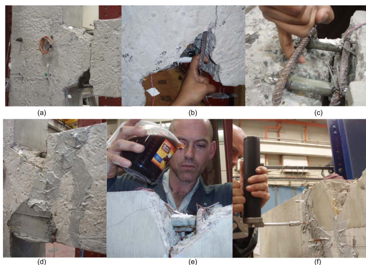
Fig. 10 Repairing of damaged JBC-2: (a) damaged concrete removed, (b) checking adequate spacing behind the bottom part of stirrup, (c) checking adequate spacing behind the top part of the stirrup, (d) sealing of the exterior face of the cracks, (e) gravity feed of epoxy adhesive in the major crack and (f) injecting epoxy adhesive using pressure-injection equipment
