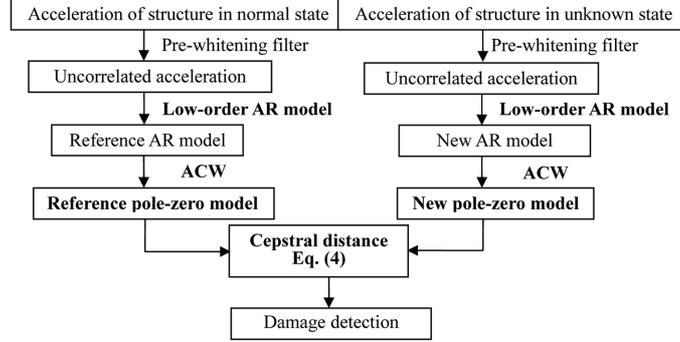
Fig. 1 Flowchart of damage detection
