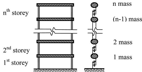
Fig. 2 Simplified structural model
