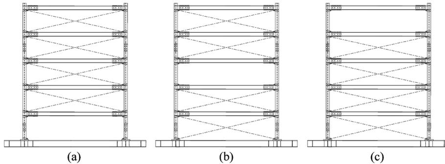
Fig. 13 Damage case: removing braces on the (a) first, (b) third and (c) fifth storey
