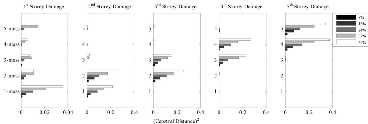
Fig. 6 Cepstral distance based on the pole-zero models (data length = 6000)
