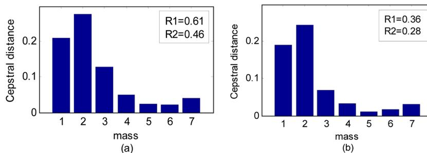
Fig. 5 7-DOF system with 24% stiffness reduction in the 2<sup>nd</sup> storey (data length = 9000, SNR = 10): (a) without ACW and (b) with ACW
