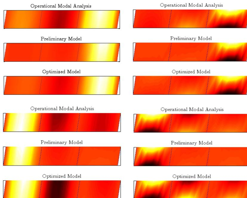
Fig. 8 Comparison of the lower-order mode shapes as measured in the experimental study, predicted in preliminary FE model, and estimated in optimized FE model. Note: FE modal vectors reduced to nodes coinciding with sensor locations to maintain consistency with experimental modes
