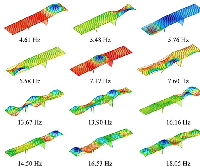
Fig. 6 FEA mode shapes and eigenfrequencies developed from preliminary model corresponding to modes identified in full-span OMA
