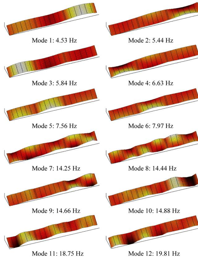
Fig. 3 Mode shapes reconstructed from first instrumentation configuration (Fig. 2(a)) with associated experimental eigenfrequency estimates. Note: Mode shape patterns limited to pure bending and first-order torsional modes due to transverse density of sensor array. Abutment and pier supports assumed to be zero displacement
