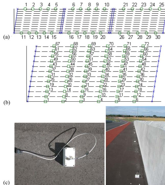
Fig. 2 Instrumentation configurations: (a) stationary vibration sensors for full-span monitoring over exterior beams, (b) reference-based dense vibration monitoring across easternmost span over all beams and (c) accelerometer and wireless sensor nodes installed on deck surfacing
