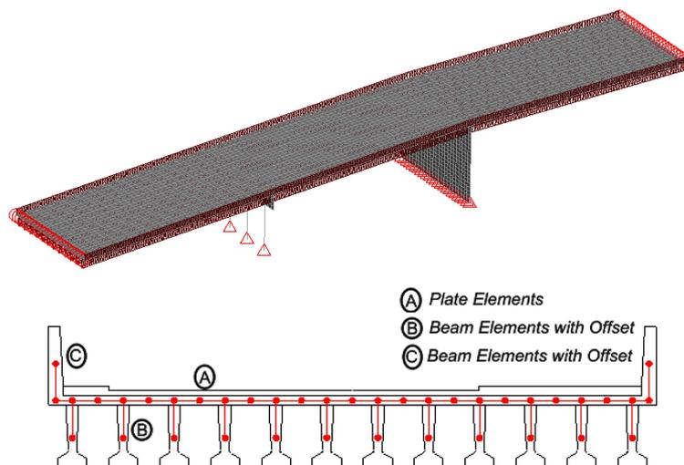
Fig. 5 Finite element model of Nine Wells Rail Bridge and cross-sectional reduction of deck, beams and parapets to plate and beam elements. Note: Preliminary FE model neglects stiffness contribution of deck surfacing, which is represented as a lumped mass proportional to the depth
