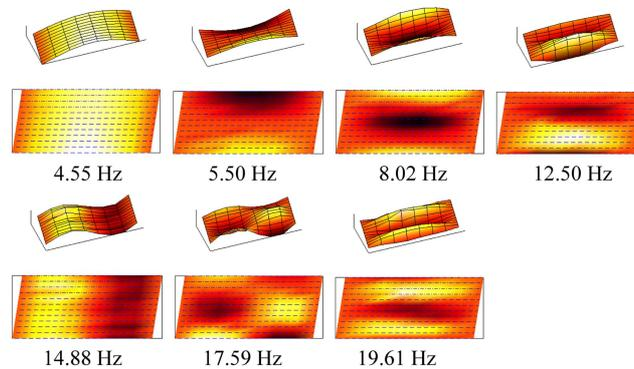
Fig. 4 Mode shapes along with associated experimental eigenfrequency estimates reconstructed for easternmost span from second instrumentation configuration (Fig. 2(b)). Note: Stochastic Subspace Identification used for OMA
