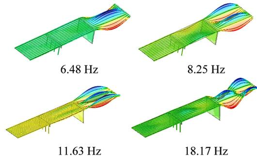
Fig. 7 Extended set of FEA mode shapes and eigenfrequencies developed from preliminary model corresponding to higher-order torsional modes on the easternmost span identified in reference-based OMA
