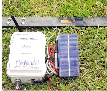
Fig. 5 Sensor node with a solar panel
