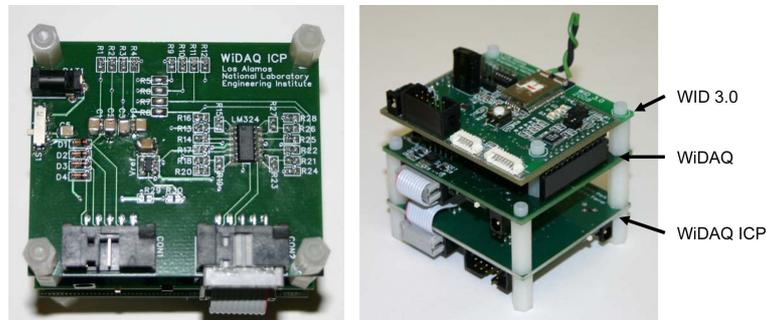
Fig. 4 WiDAQ IPC (left) and assembled modules for vibration data acquisition (right)
