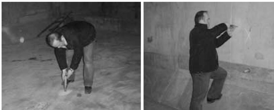
Fig. 12 Some views of the measurements using Schmidt hammer
