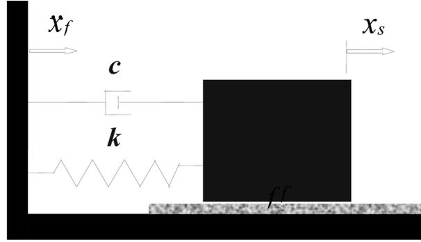
Fig. 1 Model of a SDOF system on the friction surface
