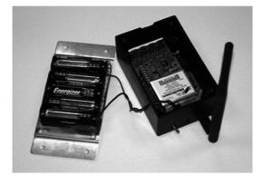
Fig. 1 Low-cost WiMMS wireless sensor proposed for structural monitoring of wind turbines
