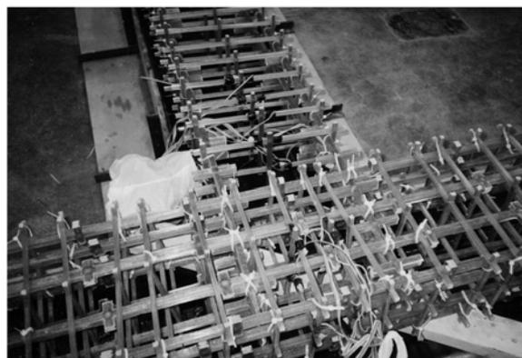
Fig. 3 View of the GFRP reinforcement cage for specimen (J4)
