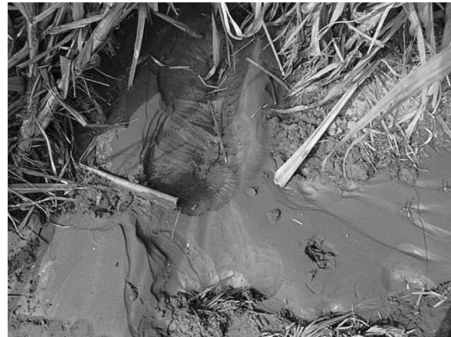
Fig. 2 Sand boils in a rice field at Jingliao following the Chiayi earthquake
