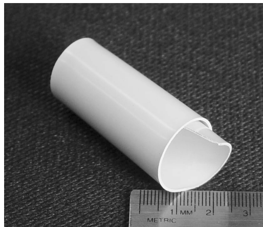
Fig. 1 Picture of flexible piezoelectric paint
