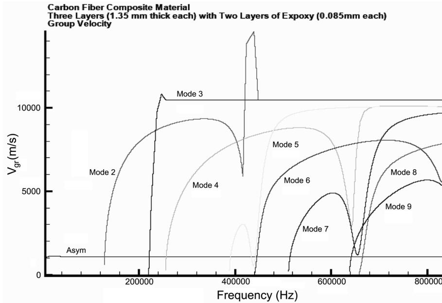
Fig. 10 Dispersion curve for carbon fiber composite plate (Group velocity) (simulated by DISPERSE, Imperial College, UK)
