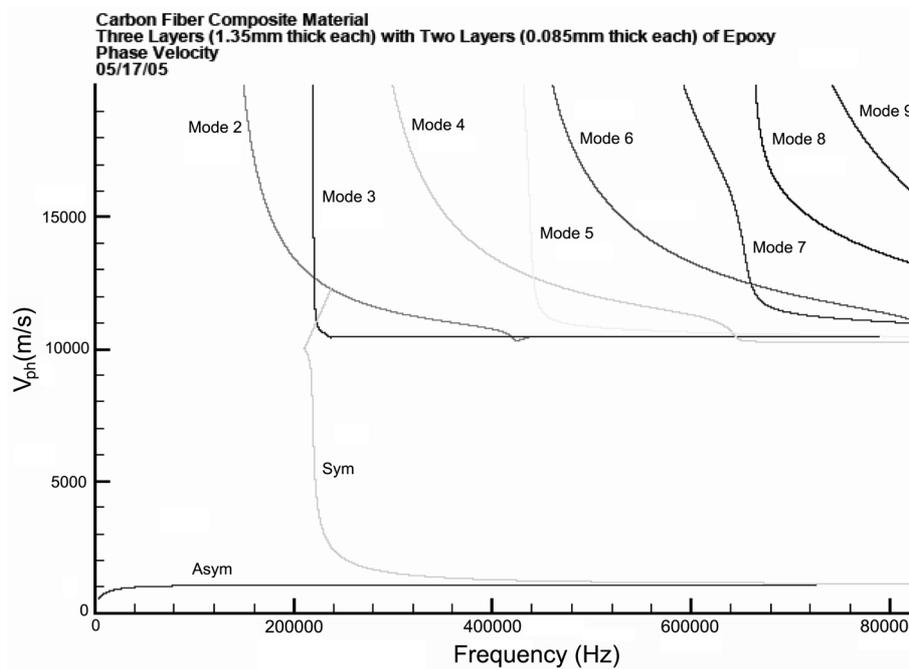
Fig. 11 Dispersion curve for carbon fiber composite plate (Phase velocity)(simulated by DISPERSE, Imperial College, UK)
