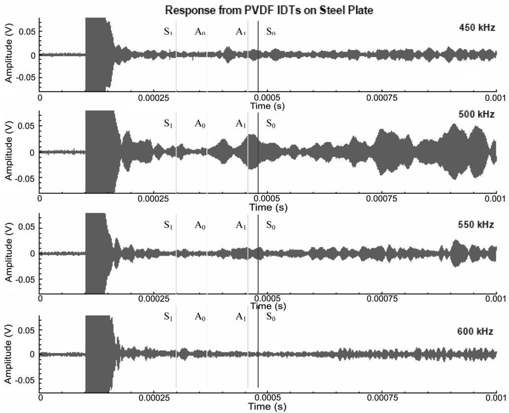
Fig. 8 Response from PVDF IDTs at different frequencies
