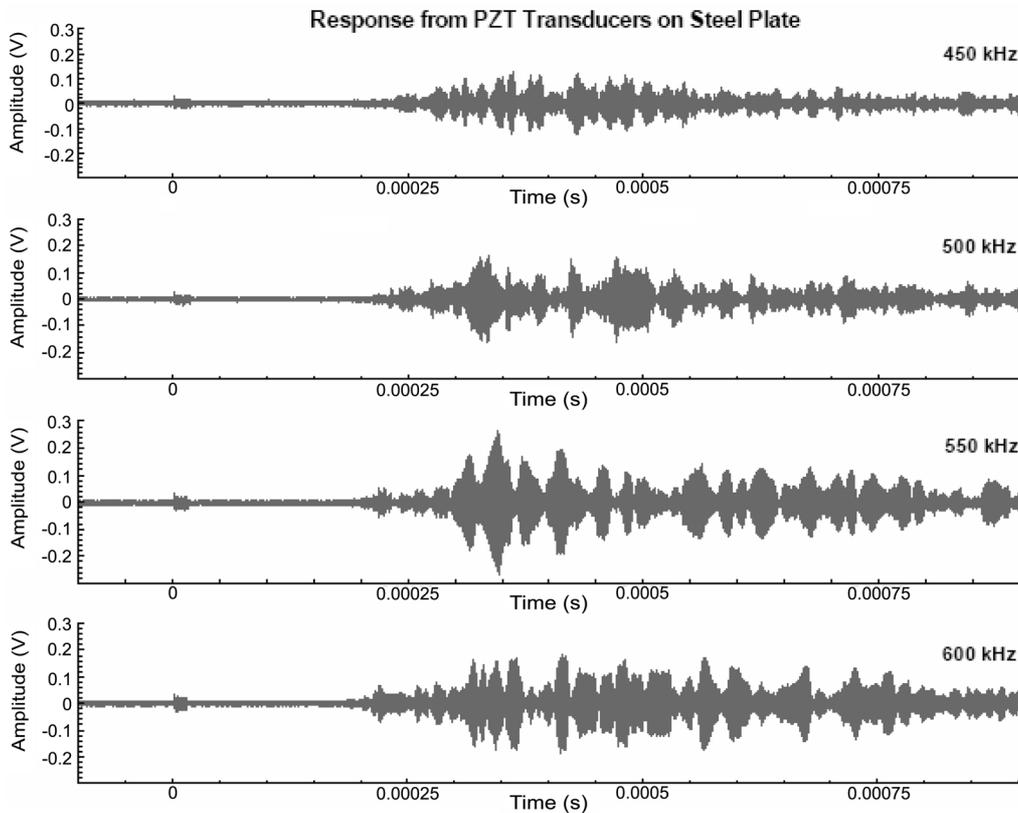
Fig. 9 Response from PZT transducers on steel plate
