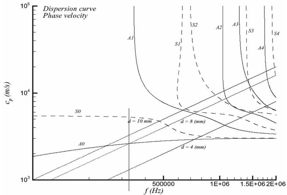
Fig. 2 Dispersion curve for steel plate (Phase velocity) (simulated by DISPERSE, Imperial College, UK)
