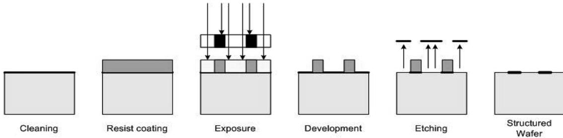
Fig. 4 Photolithography technology for building PVDF IDTs
