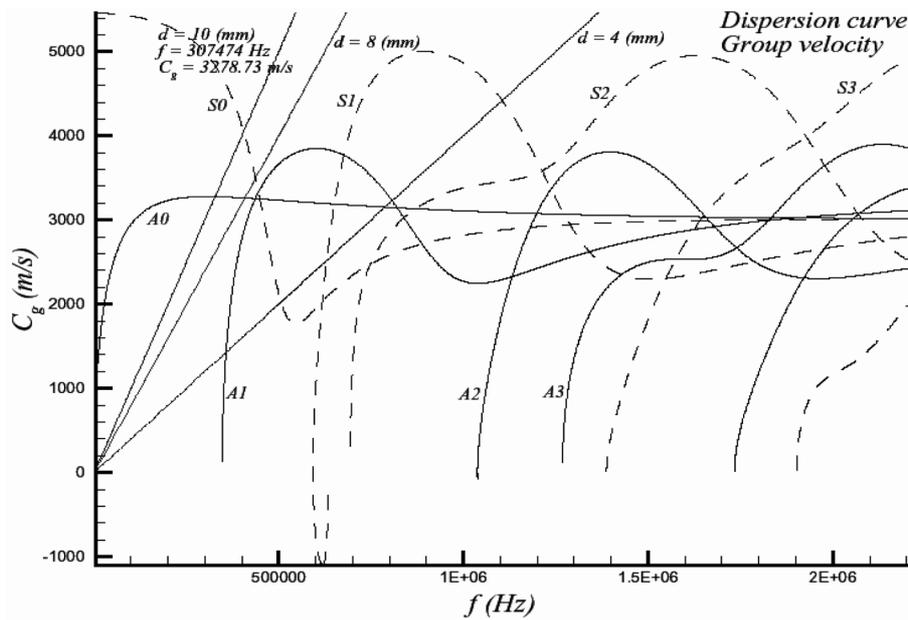
Fig. 3 Dispersion curve for steel plate (Group velocity) (simulated by DISPERSE, Imperial College, UK)
