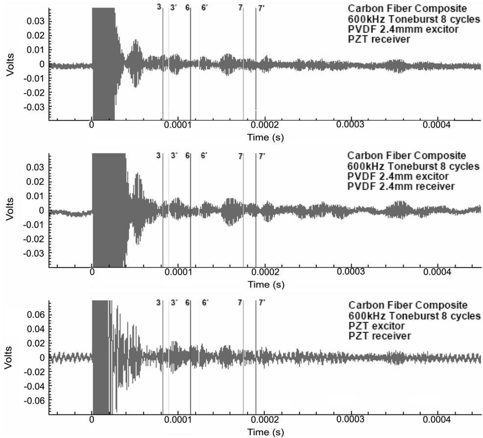
Fig. 13 Comparison between PVDF IDTs and PZT transducers on carbon fiber composite plates at 600 kHz
