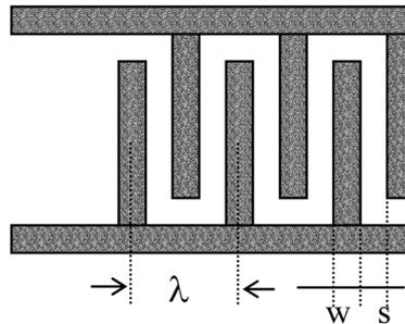
Fig. 1 Sketch of transducer electrodes
