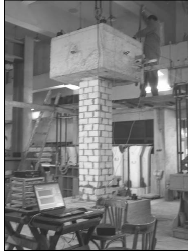
Fig. 6 The 1/16 th scale model minaret tested at the concrete research laboratory, Cairo university
