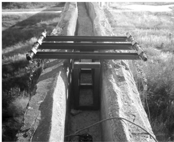
Fig. 5 Rigid base to support the upper end of the SMA prestressing assembly
