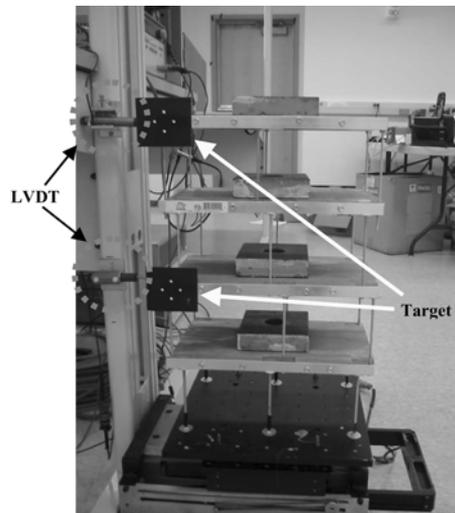
Fig. 8 A shear building model
