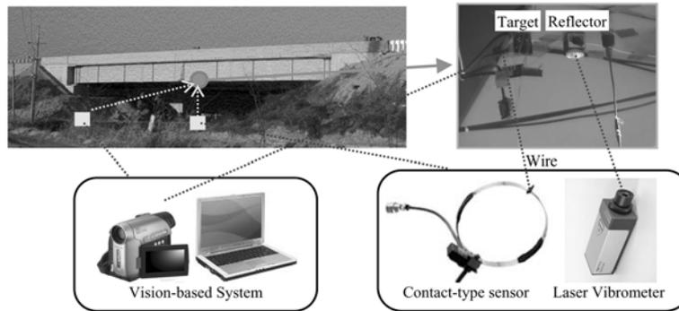
Fig. 2 Test setup on a target bridge
