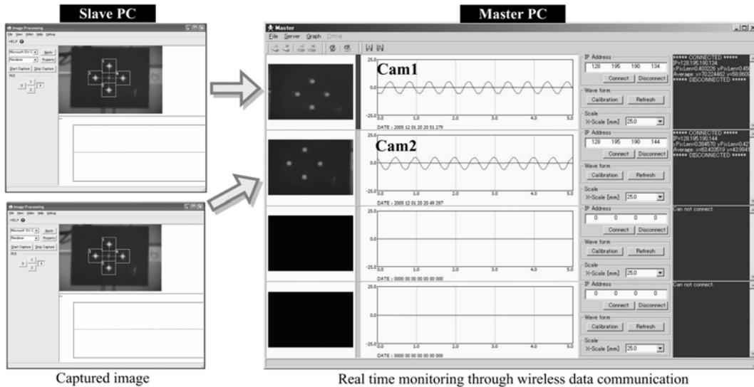
Fig. 5 Display windows of vision-based multi-points measurement system
