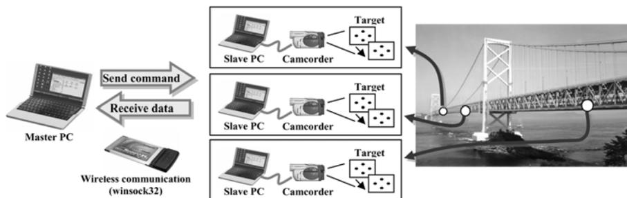
Fig. 4 Vision-based multi-points measurement system
