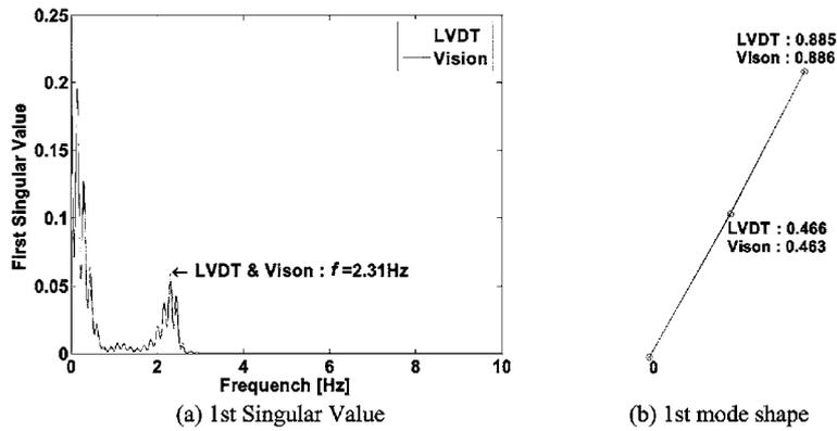
Fig. 10 Modal parameter identification using frequency domain decomposition technique
