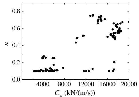
Fig. 8 Pareto optimal solutions to the parameters of the viscous dampers
