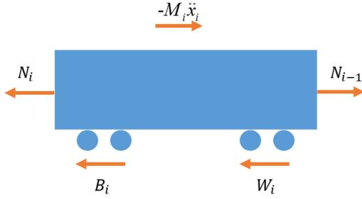
Fig. 2 Dynamic model of a unit of train in the longitudinal direction
