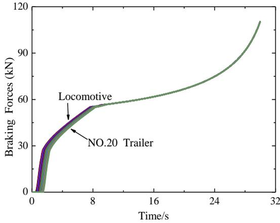
Fig. 3 Time history of braking forces (initial braking speed= 80 km/h)
