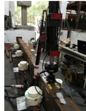
(c) Hydraulic actuator at the midspan
