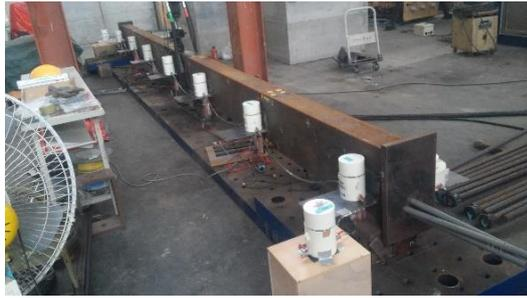
(a) Test rig of the static tests
