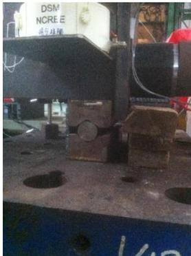
(a) Hinge support used for pinned-end constraints
