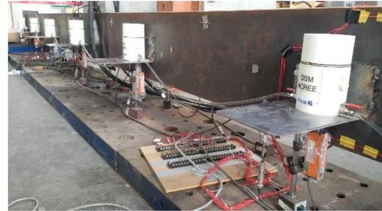
(b) FBG–DSM sensors and dial indicators along the beam's length
