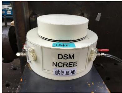
(b) Reference FBG–DSM sensor at one beam end
