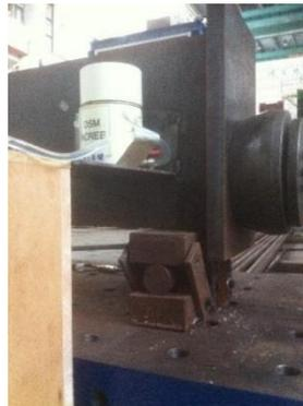
(b) Roller support used for pinned-end constraints
