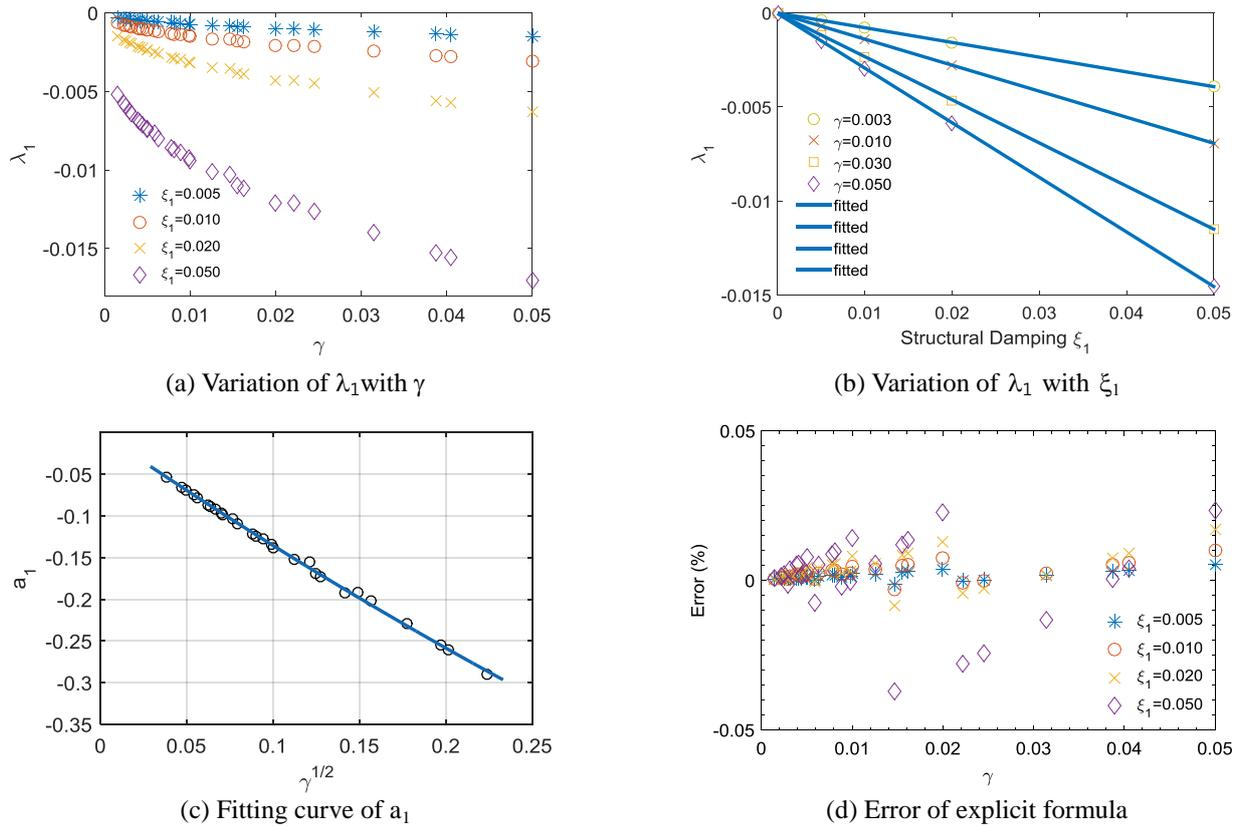
Fig. 4 Curve fitting of optimal tuning ratio
