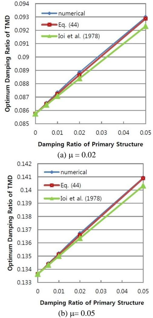
Fig. 7 Comparison of optimal damping of a TMD under harmonic excitation
