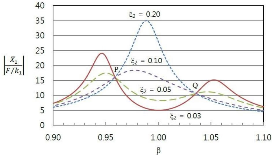
Fig. 2 Steady state response of structure with LCVA installed under harmonic forced motion ( $\mu=0.02$ ,  $\lambda=1$ ,  $r_A =0.8$ ,  $r_A=0.5$ )
