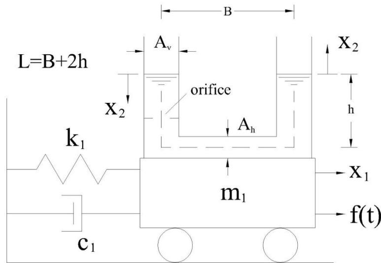
Fig. 1 Liquid column vibration absorber
