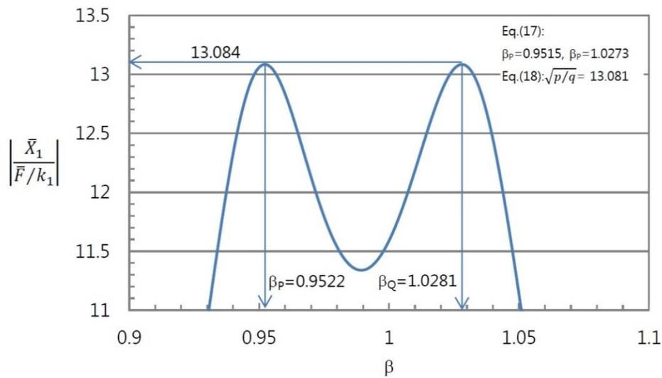
Fig. 3 Steady state response of structure with optimum LCVA installed ( $\mu=0.02$ ,  $r_A =0.8$ ,  $r_A=0.5$ ,  $\lambda=0.9844$ ,  $\xi_2=0.0660$ )
