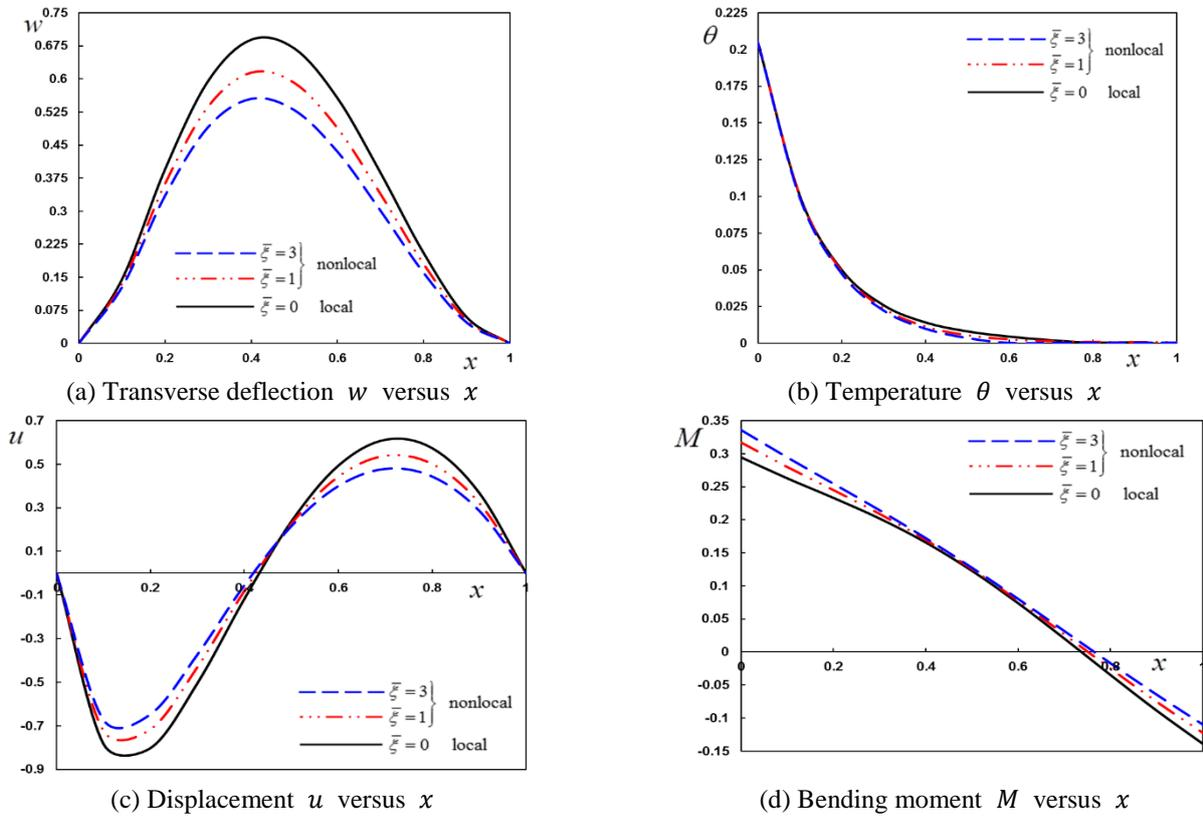
Fig. 3 The transverse deflection, temperature, displacement and thermal stress distributions of the nanobeam for different values of the nonlocal thermoelastic parameters  $\xi$
