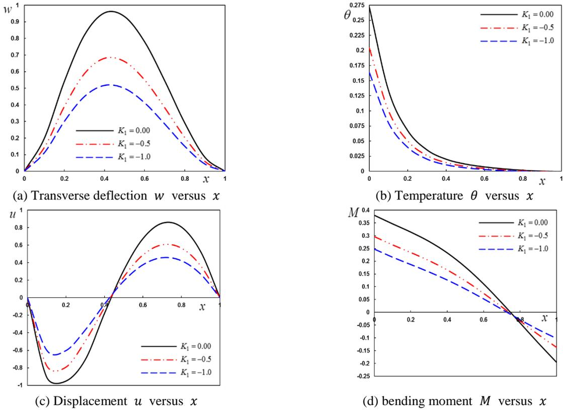
Fig. 2 The transverse deflection, temperature, displacement and thermal stress distributions of the nanobeam for different values of the variability thermal conductivity parameter  $K_1$ .
