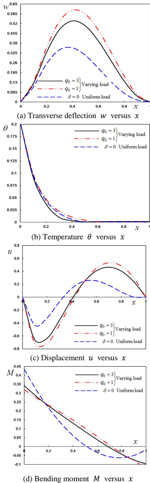
Fig. 5 The transverse deflection, temperature, displacement and thermal stress distributions of the nanobeam for different values of the the point load  $q_0$
