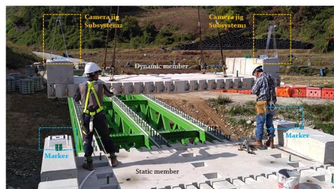
Fig. 21 Setting camera jigs and markers
