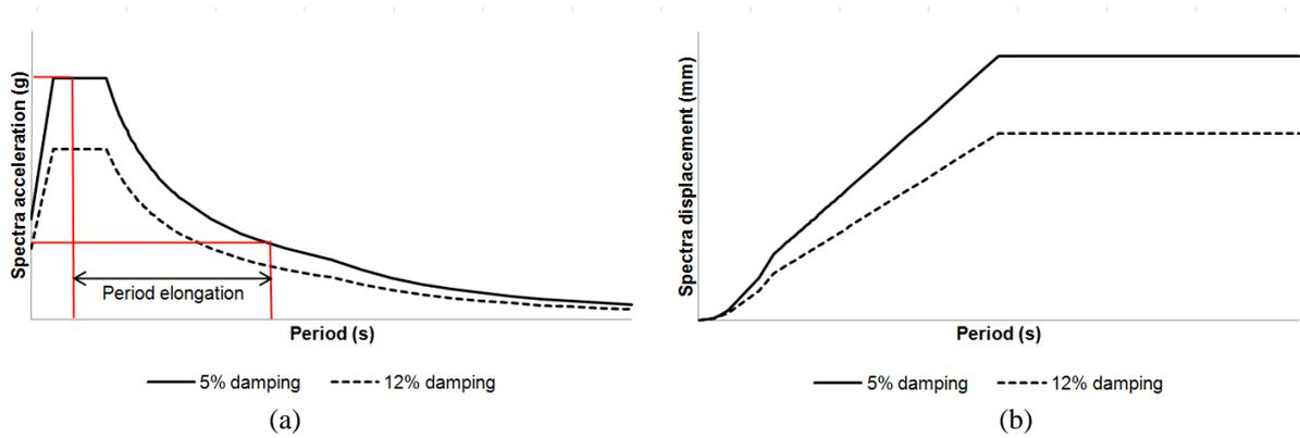
Fig. 1 Period Elongation of Base-Isolated Structure in (a) Acceleration and (b) Displacement Spectra
