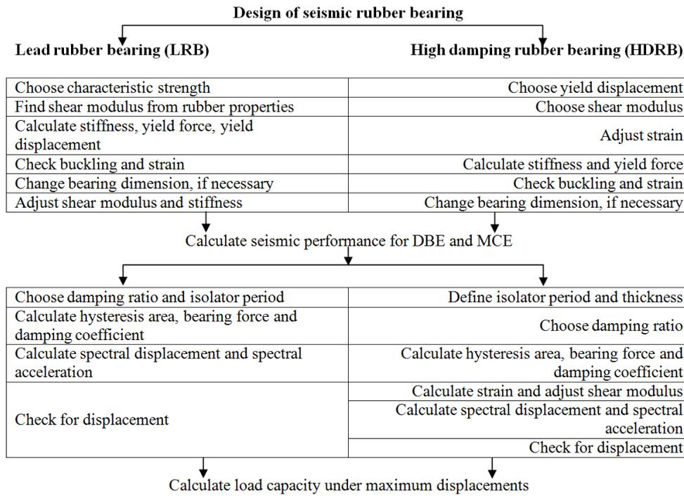
Fig. 2 General design steps of HDRB (modified from Islam *et al.* 2011)
