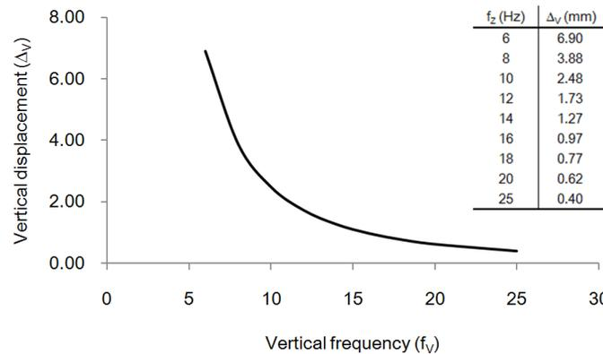
Fig. 3 Plot of vertical frequency as a function of vertical displacement
