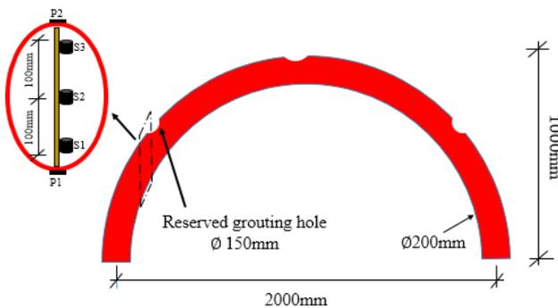
Fig. 5 Dimensions of the steel tube specimen and the location of the transducers
