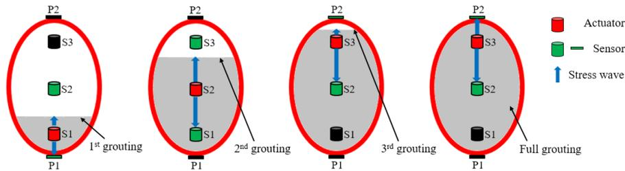
Fig. 3 Detection schematic of active sensing based grouting compactness monitoring
