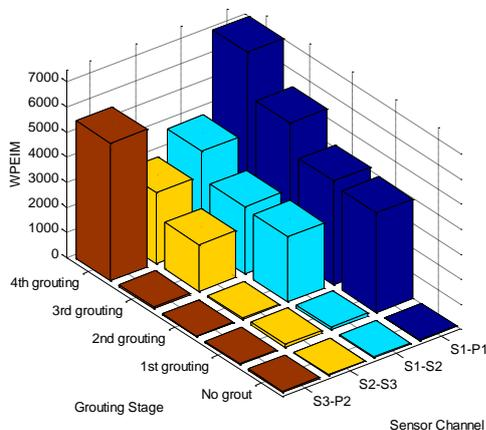
Fig. 8 Results of WPEIM-Vertically distributed sensor channels: S1-P1, S1-S2, S2-S3, S3-P2
