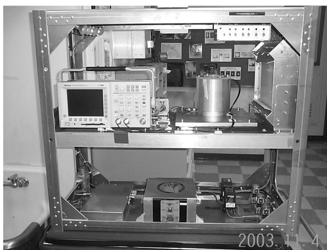
Fig. 13 Assembly of test setup on the drop tower rig at NASA Glenn
