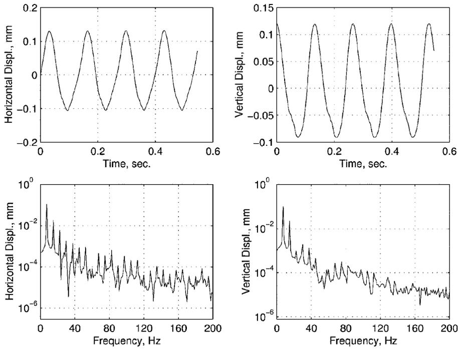
Fig. 3 Dynamic behaviour of a crack shaft at 450 RPM
