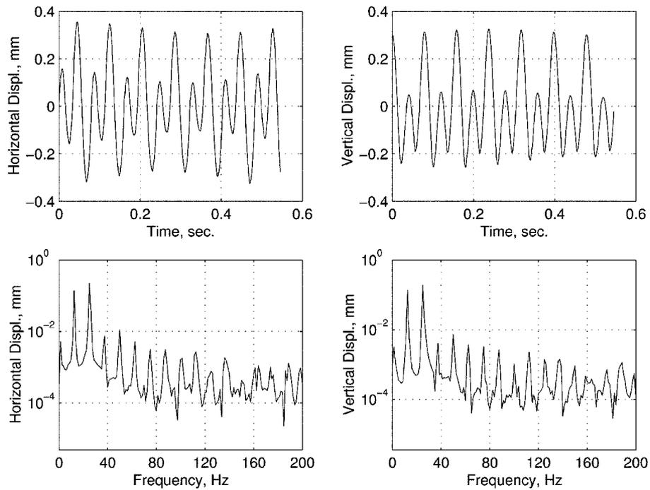
Fig. 7 Dynamic behaviour of a crack shaft at 750 RPM
