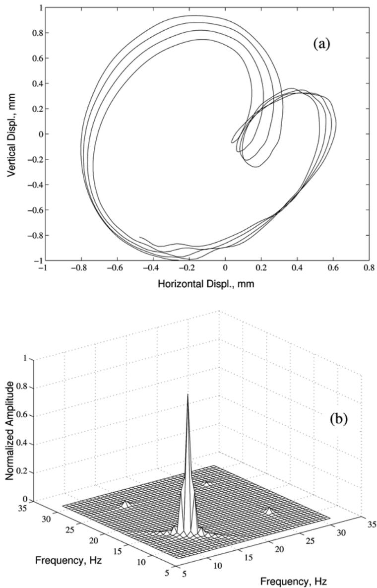
Fig. 12 Simulated dynamic behaviour of a crack shaft ((a) Orbit plot, (b) Bi-spectrum)
