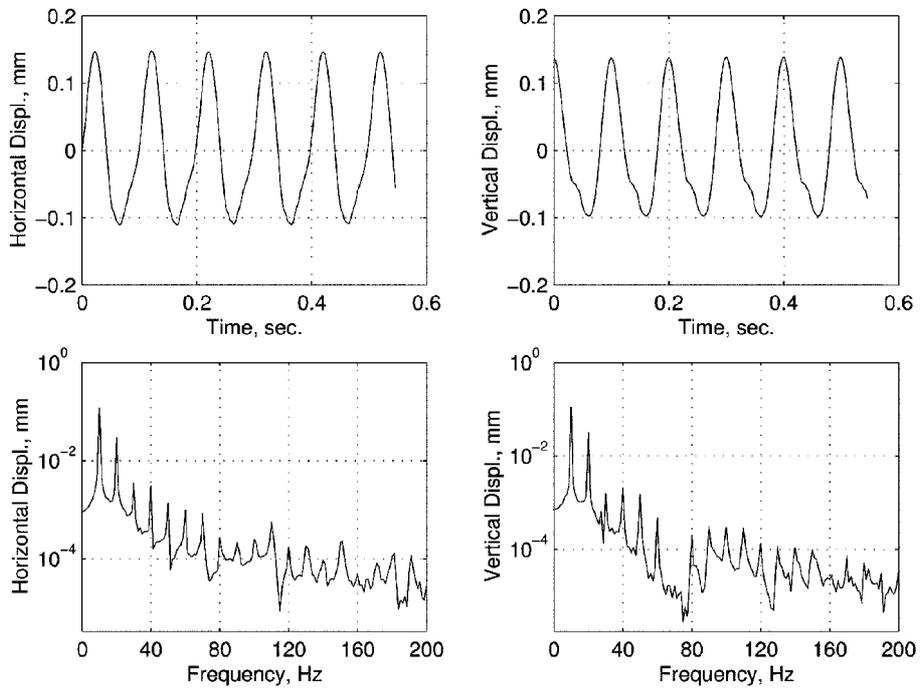
Fig. 4 Dynamic behaviour of a crack shaft at 600 RPM
