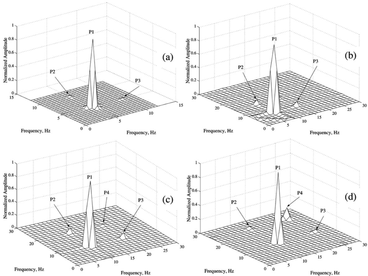
Fig. 9 Bi-spectra of a cracked shaft response in vertical direction
