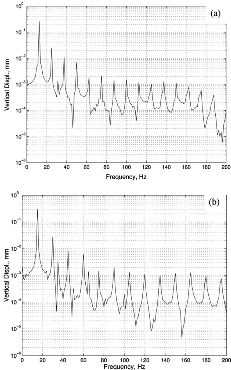
Fig. 10 Spectra of a misaligned shaft response in vertical direction ((a) 750 RPM, (b) 900 RPM)
