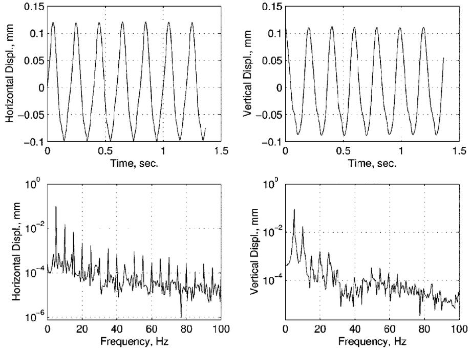
Fig. 2 Dynamic behaviour of a crack shaft at 300 RPM
