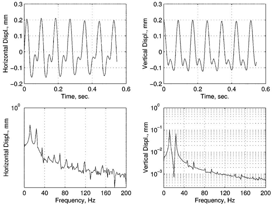
Fig. 6 Dynamic behaviour of a crack shaft at 700 RPM
