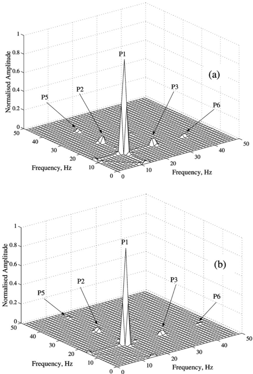
Fig. 11 Bi-spectra of a misaligned shaft response in vertical direction ((a) 750 RPM, (b) 900 RPM)
