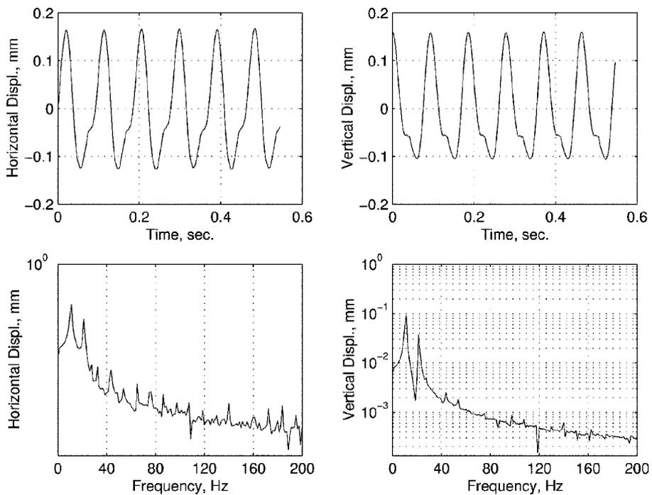
Fig. 5 Dynamic behaviour of a crack shaft at 650 RPM
