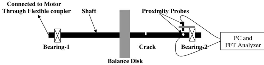
Fig. 1 Schematic of the experimental rig
