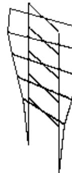
(a) 1st torsional mode (T1, 1.07 Hz)
