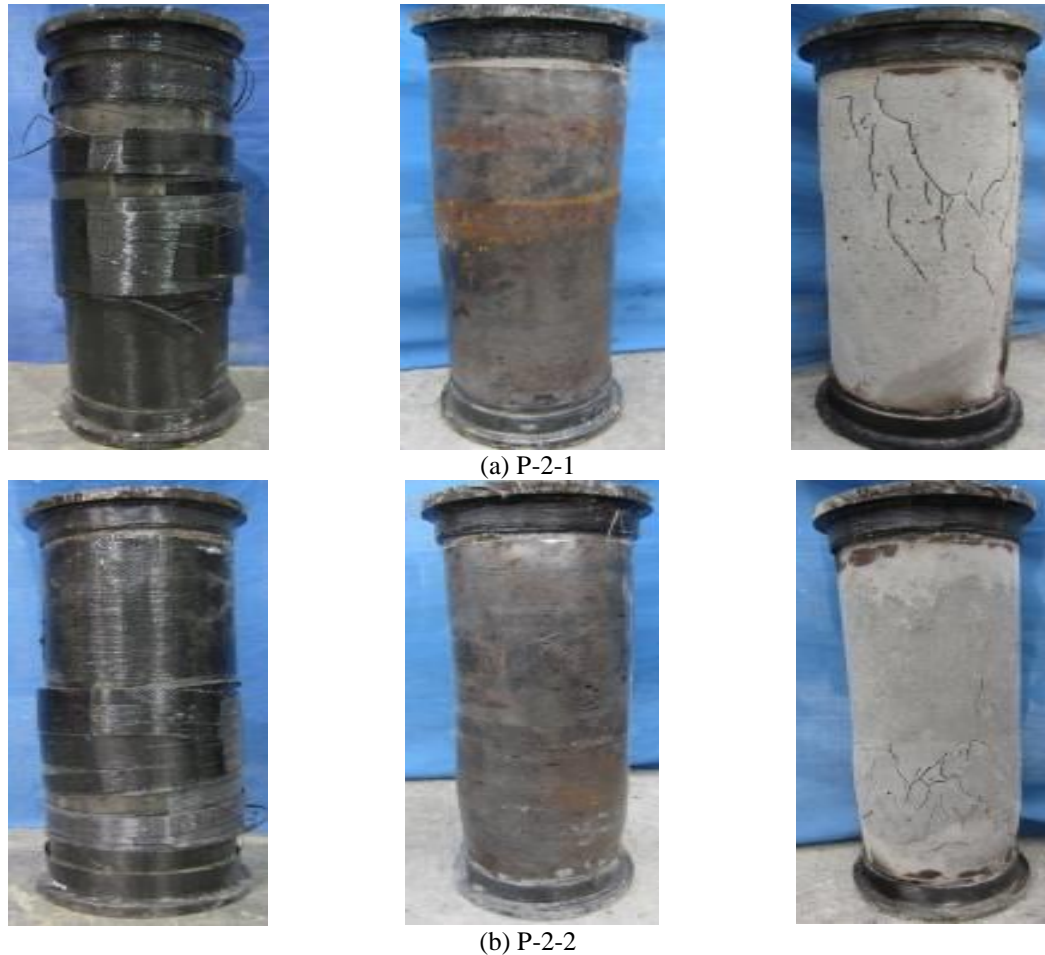
Fig. 6 Final failure images of specimens
