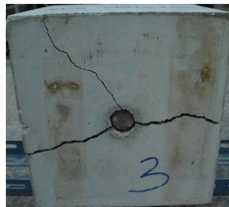
(b) Concrete splitting failure
