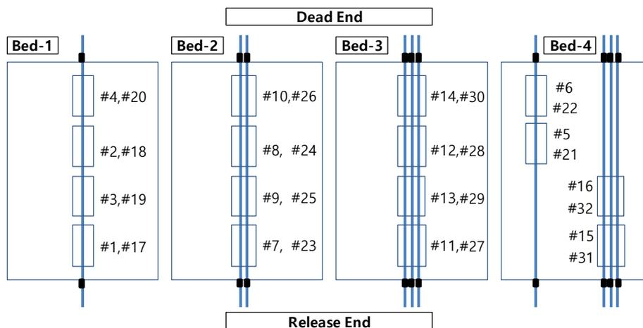
Fig. 3 Prestressing beds and fabrication scheme for test specimens
