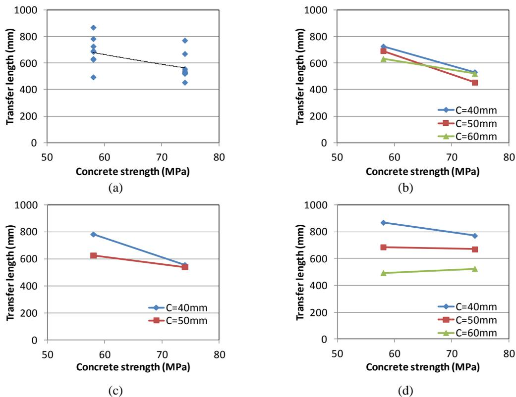
Fig. 5 Transfer length according to the concrete compressive strength: (a) All, (b) No. of PS strands = 1, (c) No. of PS strands = 2 and (d) No. of PS strands = 3
