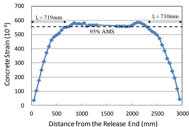
Fig. 4 Refined strain measurement and determination of transfer length (#1)
