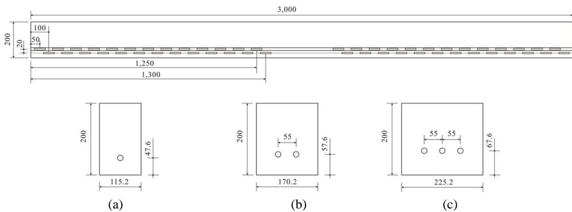
Fig. 1 Details of test specimens and attached locations of strain gauges: (a) #1, #2, #17, #18, (b) #9, #10, #25, #26; and (c) #15, #16, #31, #32
