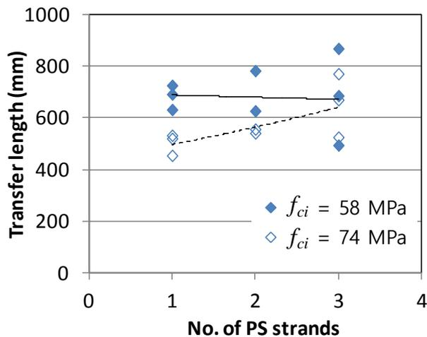
Fig. 8 Variation in transfer length according to the number of PS strands
