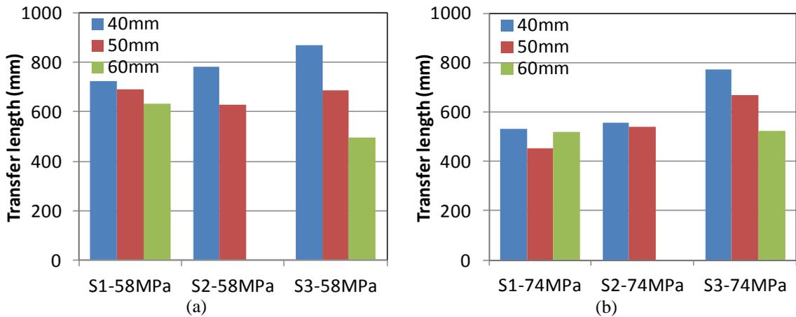
Fig. 7 Transfer length according to the concrete cover depth and the number of PS strands (S1: 1 PS strand; S2: 2 PS strands; S3: 3 PS strands): (a) concrete compressive strength of 58 MPa and (b) concrete compressive strength of 74 MPa
