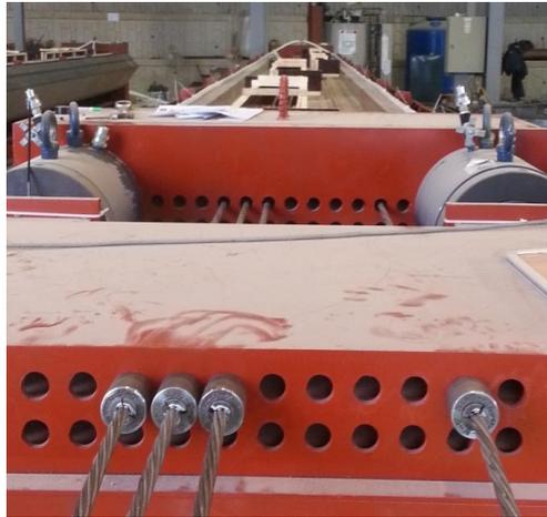
Fig. 2 Fabrication of pretensioned prestressed concrete beams on Bed-4
