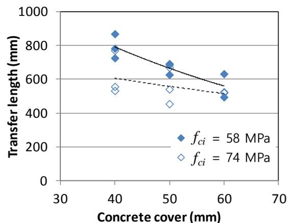
Fig. 6 Transfer length according to the concrete cover depth
