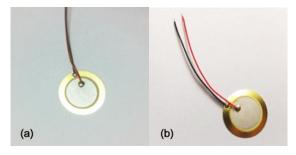
Fig. 1 PZT senor (a) before coating and (b) after coating with acrylic resin
