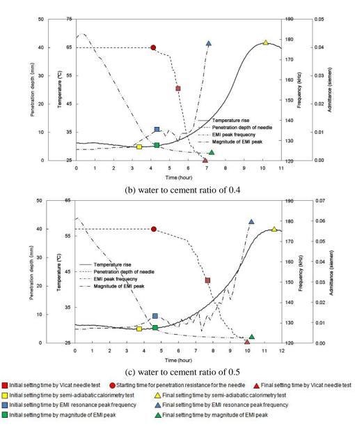
Fig. 9 The setting times by various testing methods
