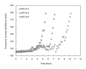
Fig. 8 EMI resonance peak frequency as function of material age
