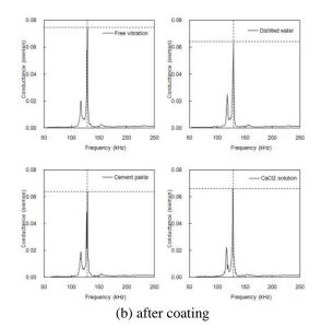
Fig. 2 EMI signatures of PZT sensor under various conditions
