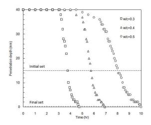
Fig. 4 Penetration depth of needle as a function of material age
