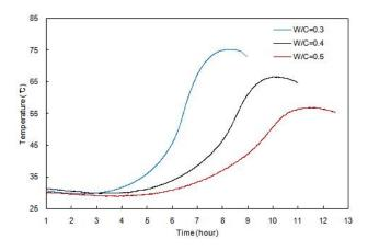
Fig. 5 Temperature of cement paste as function of material age
