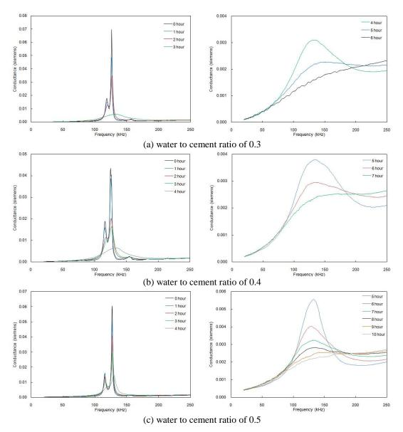
Fig. 6 EMI signatures of PZT sensor embedded in cement pastes
