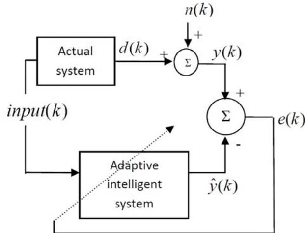
Fig. 1 System modelling using an adaptive intelligent system (Mohammadhassani 2013a)
