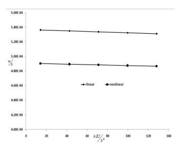
Fig. 6 Comparison between linear and nonlinear dimensionless transverse displacement in terms of dimensionless stiffness parameter
