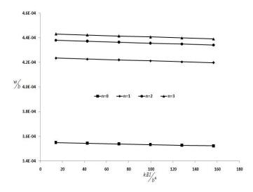
Fig. 2 The distribution of dimensionless transverse displacement in terms of dimensionless stiffness parameter for different non-homogenous indexes
