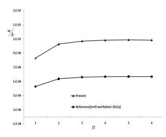
Fig. 11 The comparison between dimensionless transverse displacement of present and previous (Arefi and Rahimi 2012) a results
