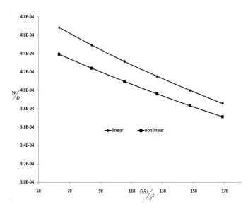
Fig. 7 Comparison between linear and nonlinear dimensionless transverse displacement in terms of dimensionless shear parameter
