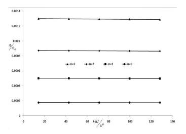
Fig. 4 The distribution of dimensionless electric potential in terms of dimensionless stiffness parameter for different non-homogenous indexes
