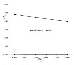
Fig. 10 The comparison between dimensionless transverse displacement of simply supported and fixed plate
