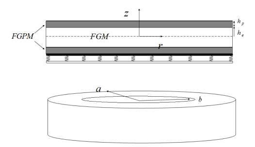
Fig. 1 FG circular plate with piezoelectric layers resting on Winkler-Pasternak foundation
