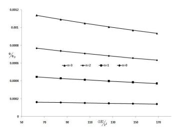
Fig. 5 The distribution of dimensionless electric potential in terms of dimensionless shear parameter for different non-homogenous indexes
