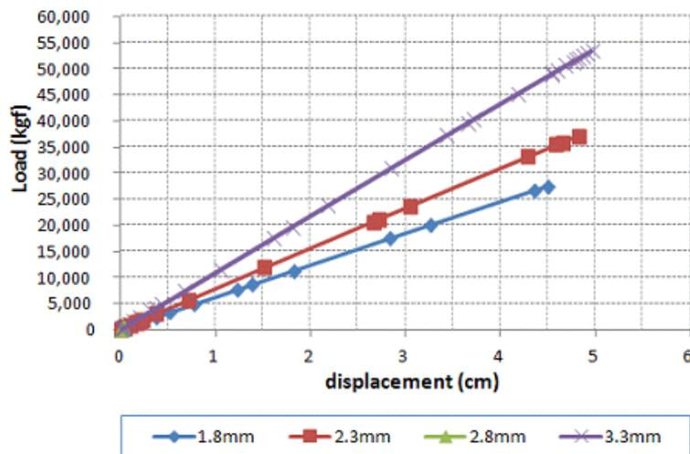
Fig. 13 Performance Comparison of Different Thicknesses (Ø48.6)
