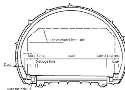
Fig. 3 Components of a road tunnel
