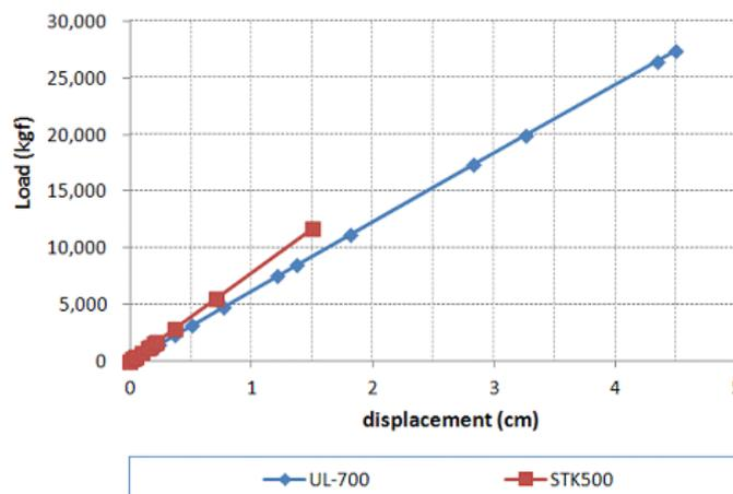
Fig. 10 Comparison between STK500 and UL-700
