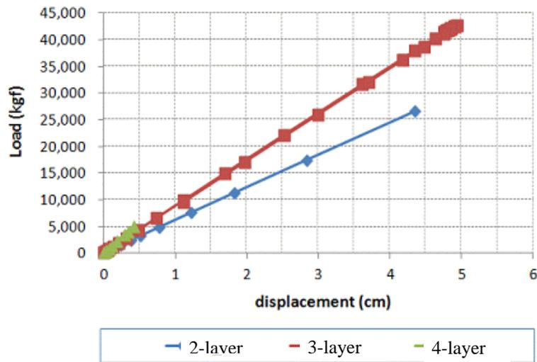
Fig. 14 Performance Comparison of a Different Number of Layers (Ø 48.6 x 1.8\_UL-700)
