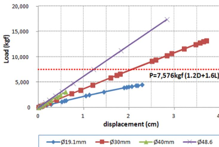
Fig. 11 Performance Comparison of Different Diameters (T=1.8 mm)
