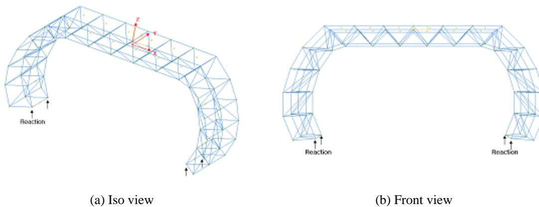
Fig. 8 Location of Reaction Points
