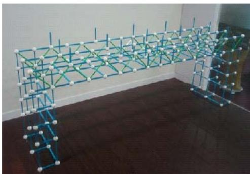
(a) Space truss frame with sharp corners
