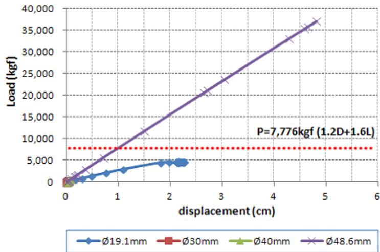
Fig. 12 Performance Comparison of Different Diameters (T=2.3mm)
