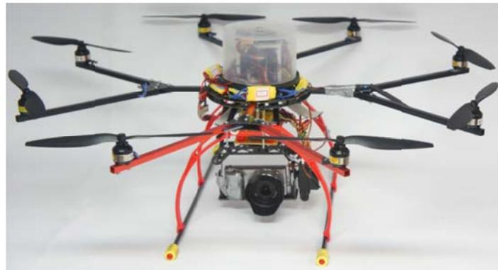
Fig. 9 Octocopter MAV system with digital camera
