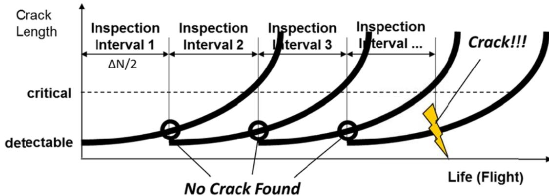
Fig. 2 The damage tolerance design principle
