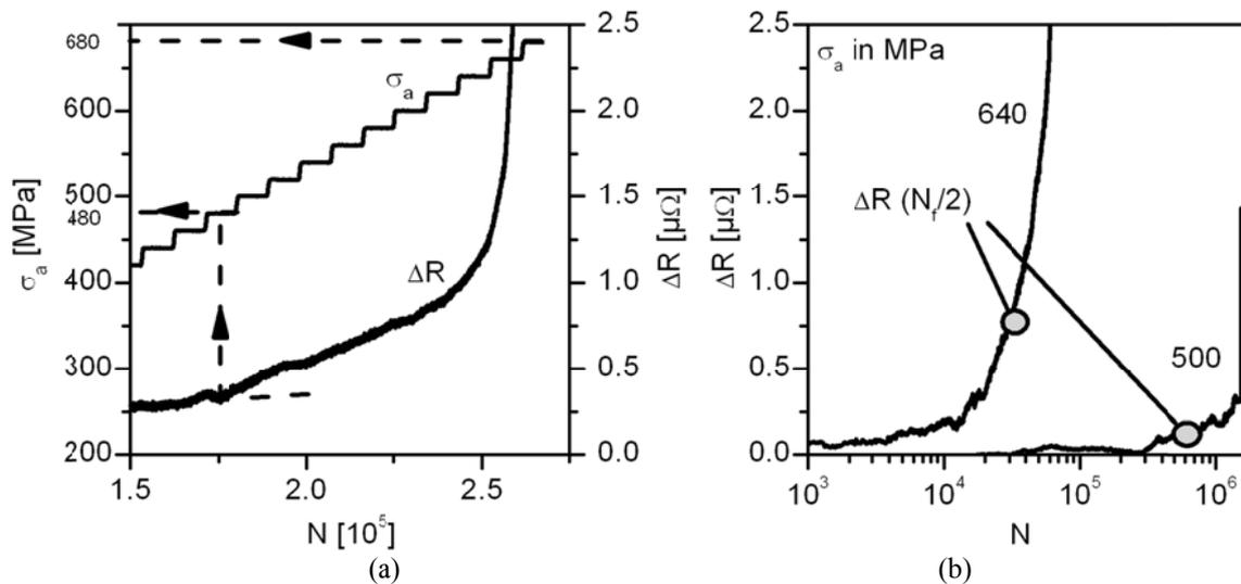
Fig. 5 Stepwise load increase test (LIT) for quenched and tempered SAE 4140 with stress amplitude  $\sigma_a$  and change in electrical resistance  $\Delta R$  related to fatigue cycles applied (a) and electrical resistance versus fatigue cycles applied at two stress levels of a constant amplitude test (b)
