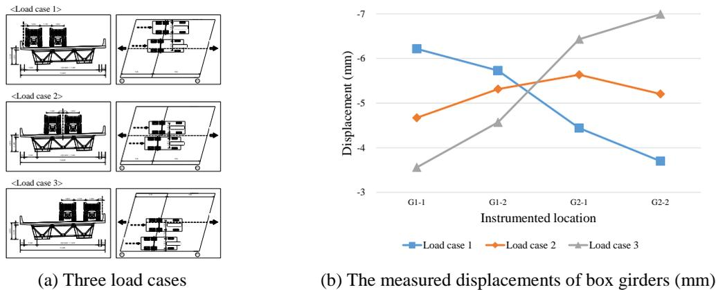
Fig. 6 Measured static displacements
