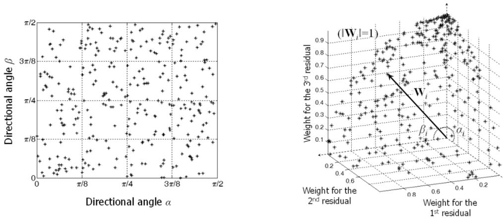
(a) Uniform sampling of two directional angles (b) Generating sets of weighting vectors
