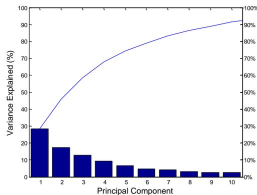
Fig. 7 Contribution of each principal component in the variance of multiple FE models
