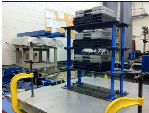
Fig. 3 A three-story steel frame structure on the uni-axial shake table at Johns Hopkins University
