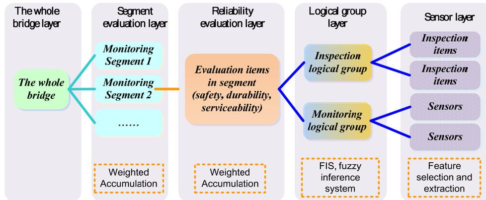
Fig. 5 The AHP based online evaluation tree of DHBHMS
