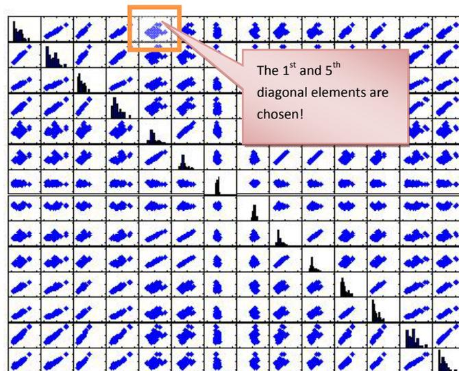
Fig. 9 Scatter plot of the diagonal element modal flexibility matrix
