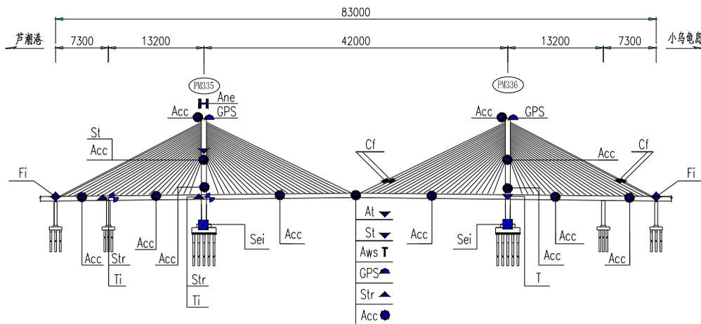
Fig. 4 The layout of the sensors on main navigation channel cable-stayed bridge At—atmosphere temperature sensor (1); St—structural temperature sensors (46); Ane—Anemometer (1); Aws—weather station (1); GPS—GPS (3); Str—FBG strain gauges (48); Acc—acceleration meter (27); Sei—strong vibration accelerometer; (2); Ti—fatigue meters (24); Fi—extension gauges (4); Cf—cable force apparatus (8)
