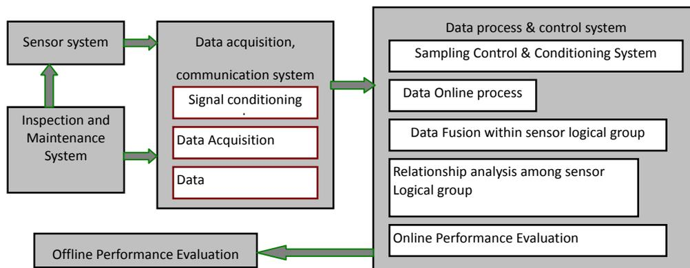
Fig. 2 The modular structure of the DHBHMS
