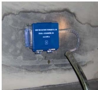
(a) Photo of the accelerate meter installed on the top panel of the girder in middle section
