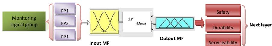
Fig. 6 The architecture of the FIS engine (Feature Pattern, abbr. FP)
