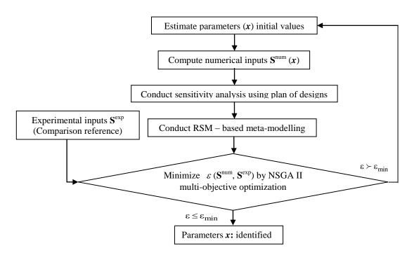
Fig. 2 Proposed behaviour/parameters' robust multi-objective identification methodology
