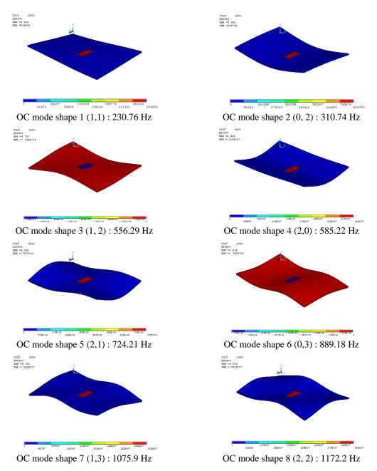
Fig. 7 Free piezoelectric adaptive plate's 8 first modes electric potential distributions
