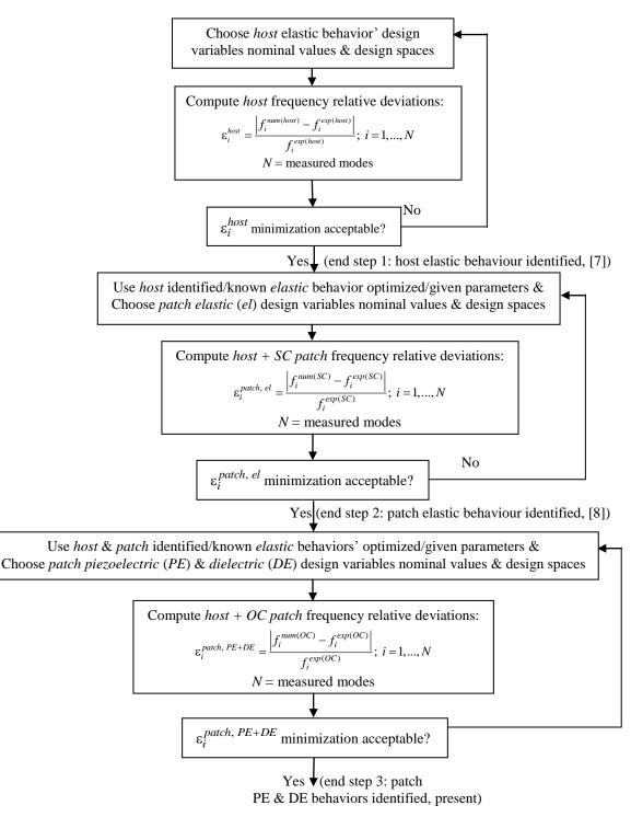
Fig. 1 Three-step frequency minimization-based materials behaviors' robust multi-objective identification ([7] Hamdi et al. 2010, [8] Hamdi et al. 2012)
