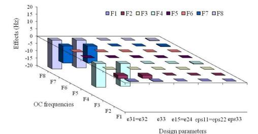
Fig. 6 Transverse isotropic behaviour 5 design parameters effects on the 8 OC frequencies
