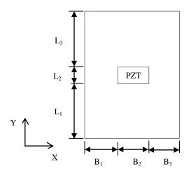
Fig. 4 Position of the patch on the plate and domains partition for the FE mesh generation
