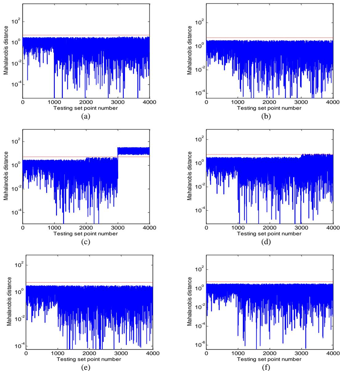
Fig. 14 Mahalanobis distances for (a) case 1, (b) case 2, (c) case 3, (d) case 4, (e) case 5 and (f) case 6 (--- Threshold value)
