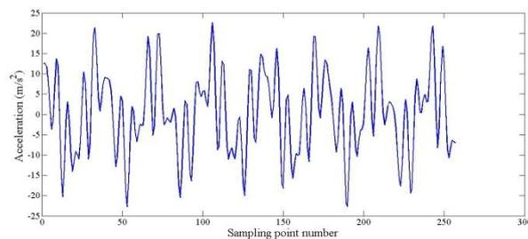
Fig. 3 Acceleration response at DOF 6
