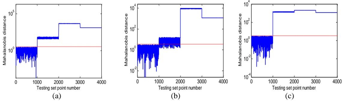
Fig. 7 Mahalanobis distances for case 2: (a) level 1 details, (b) level 2 details and (c) level 3 details (--- Threshold value)
