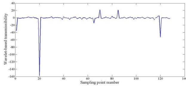
Fig. 4 Wavelet-based transmissibility between DOF 5 and 6 for healthy data (at level 1)
