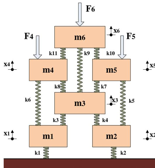
Fig. 1 6-DOF mass-spring system
