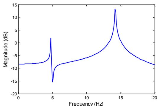
Fig. 12 Transmissibility function for healthy data
