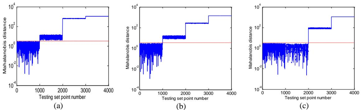
Fig. 9 Mahalanobis distances for case 4: (a) level 1 details, (b) level 2 details and (c) level 3 details (--- Threshold value)
