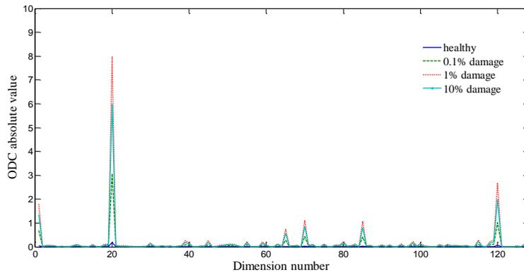
Fig. 5 Averaged outlier-displaying component for wavelet transmissibility
