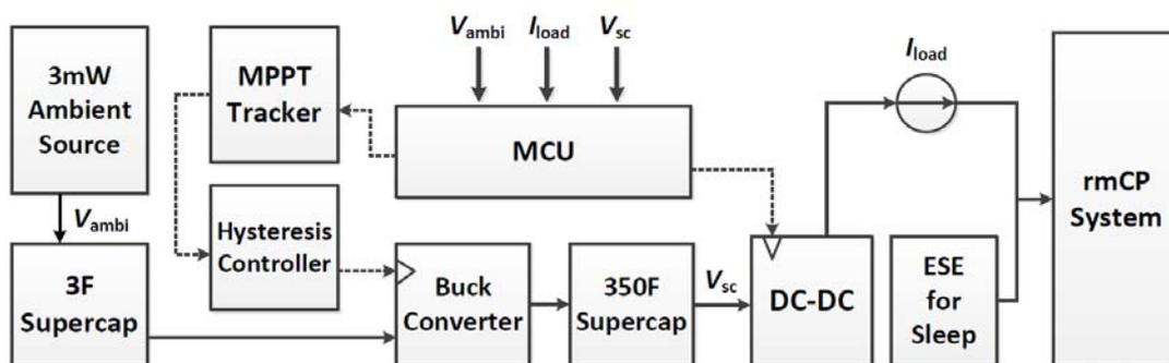
Fig. 3 System block diagram for an ultra-low power consumption harvester
