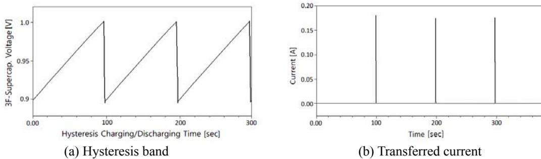
Fig. 6 Hysteresis operation during charging phase
