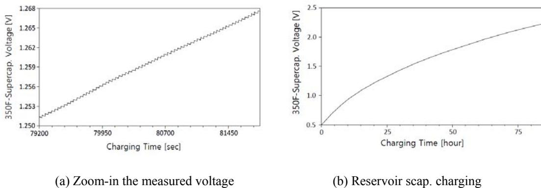
Fig. 7 Measured Charging Voltage of 350F
