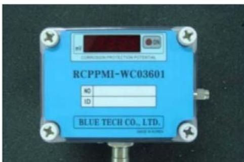
(a) Corrosion monitoring node
