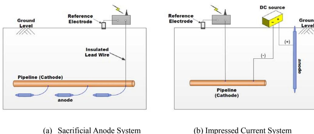
Fig. 1 Remote Corrosion Monitoring (RCM) Systems
