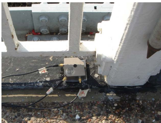
(a) Accelerometer mounted on the deck
