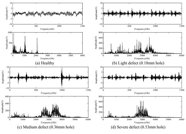
Fig. 6 Vibration signals of bearings under different levels of damage (Speed: 1,772 rpm, Load: 1 hp)
