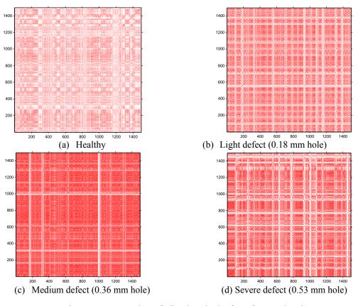
Fig. 7 Recurrence plots of vibration signlas from four test bearings (Speed: 1,772 rpm, Load: 1 HP)
