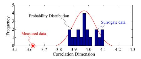
Fig. 4 Null hypothesis test result indicating a system being inherently nonlinear
