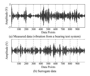
Fig. 2 Measured data and examplary surrogate data used in non-linearity test
