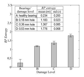
Fig. 9 RP entropy of vibration signlas from four test bearings (Speed: 1,750 rmp; Load: 2HP)
