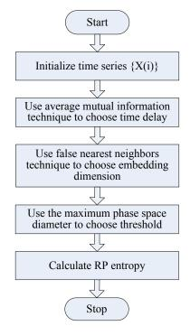
Fig. 5 Flow chart of recurrence plot entropy calculation
