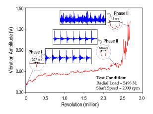
Fig. 10 Amplitude as a function of bearing revolution
