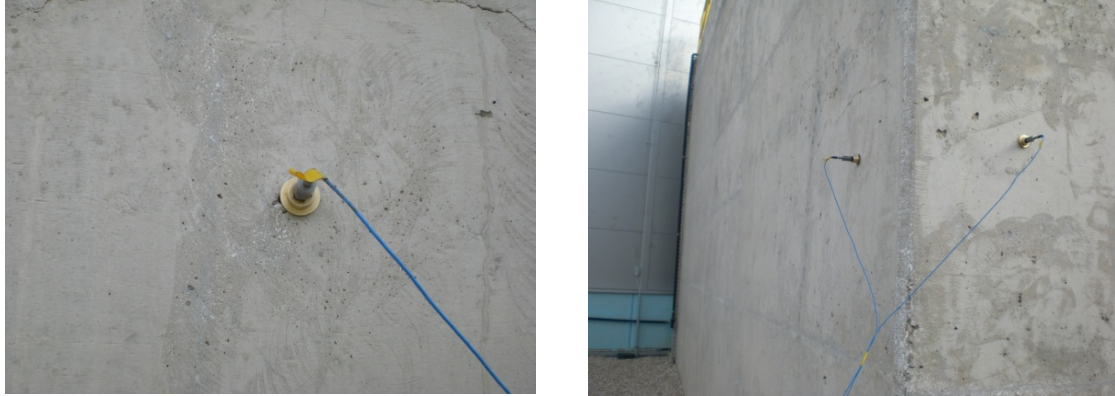
Fig. 3 A photo of field acceleration measurements
