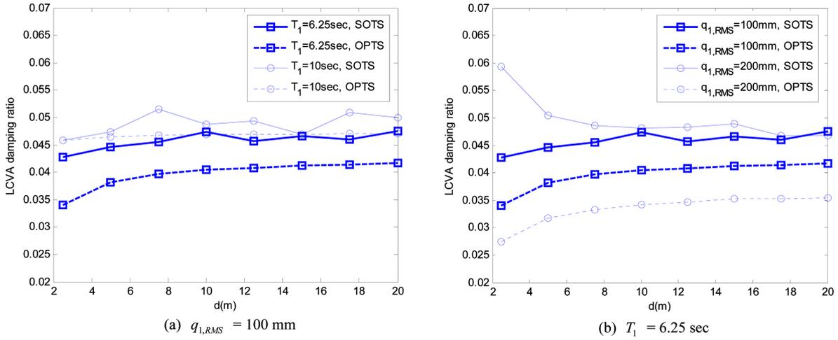
Fig. 6 Equivalent linear damping ratio of the suboptimally and optimally tuned LCVAs
