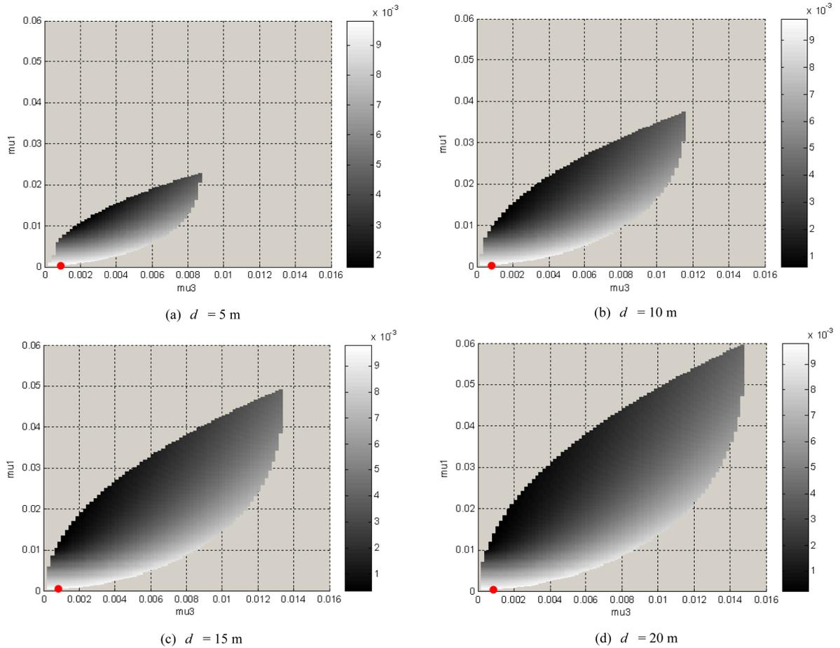
Fig. 3 Mass ratio of the horizontal liquid column over the primary structure (a,b) ( $T_1 = 6.25$  sec,  $\sigma_{q_1} = 100$  mm), (c,d) ( $T_1 = 6.25$  sec,  $q_{1,RMS} = 100$  mm)
