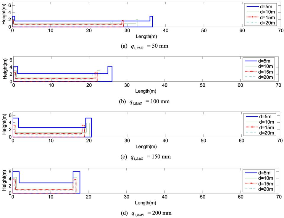
Fig. 10 Optimal shape of the LCVA ( $T_1 = 6.25$  sec)
