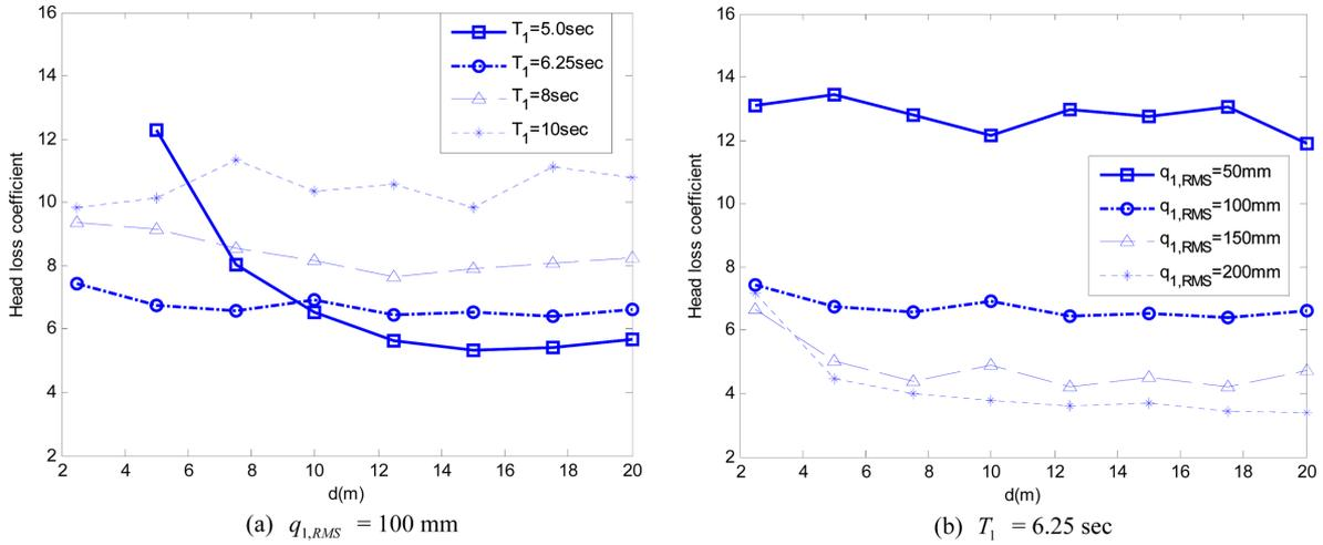
Fig. 8 Head loss coefficient of the optimal LCVA
