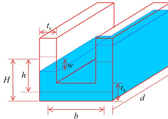
Fig. 1 Dimensions of the LCVA
