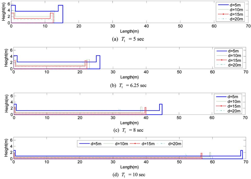
Fig. 9 Optimal shape of the LCVA ( $q_{1,RMS} = 100$  mm)
