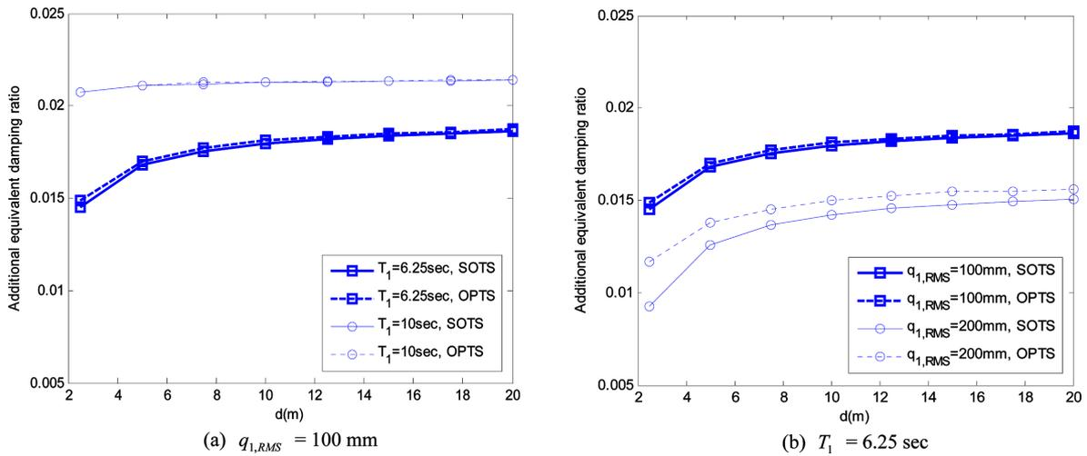
Fig. 7 Additional equivalent damping ratio achieved by the SOTS and OPTS
