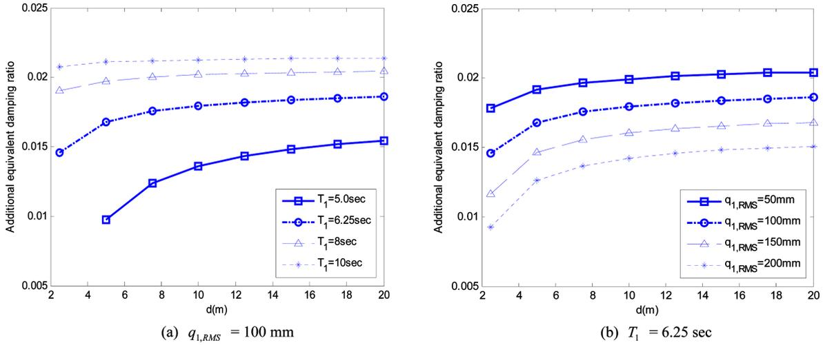
Fig. 4 Global optimal additional equivalent damping ratio
