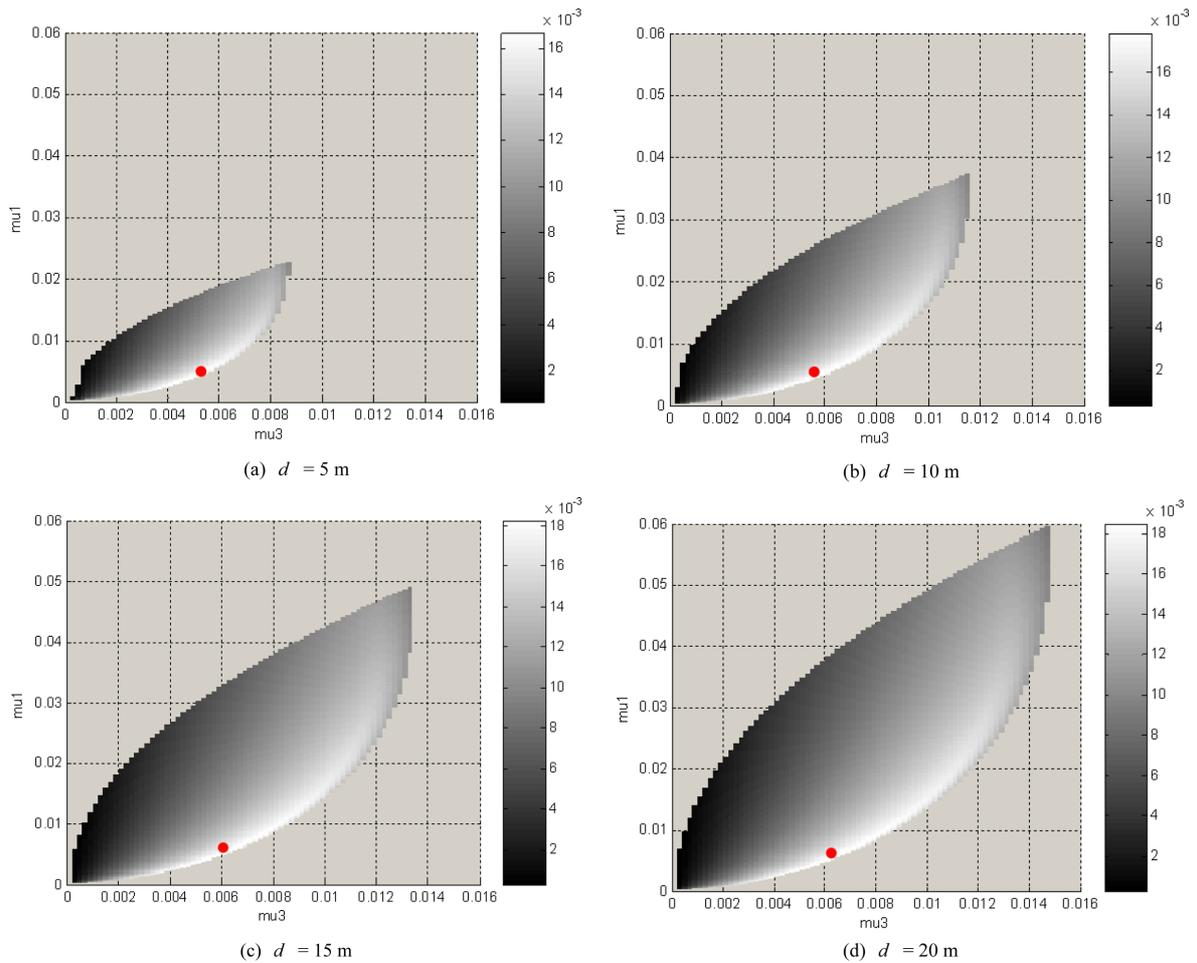
Fig. 2 Additional equivalent damping ratio ( $T_1 = 6.25$  sec,  $q_{1,RMS} = 100$  mm)
