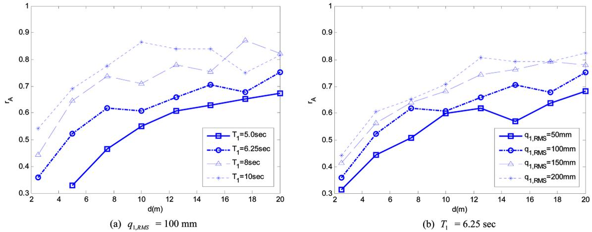
Fig. 11 Cross sectional area ratio  $r_A$  of the optimal LCVA
