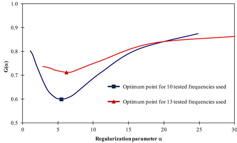
Fig. 5 The GCV as a function of Tikhonov regularization parameter  $\theta$  for cases with 10 and 13 measured frequencies adopted for updating, giving optimum regularization parameters
