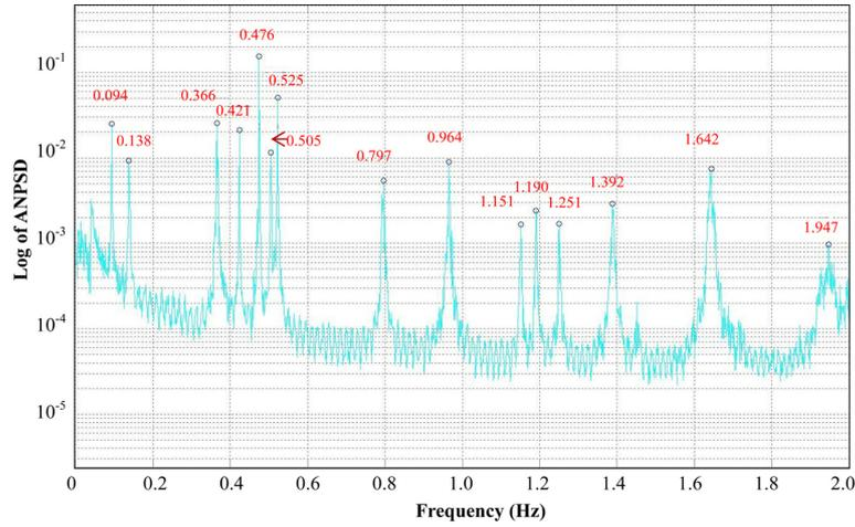
Fig. 2 Averaged normalized power spectral densities (ANPADs) of the measured acceleration data used for the Peak Picking (PP) technique
