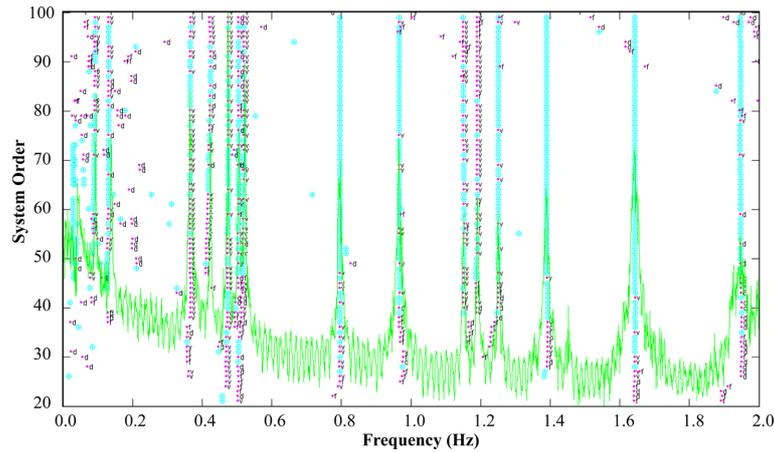
Fig. 3 The stabilization diagram of measured acceleration data used for the Stochastic Subspace Identification (SSI) technique
