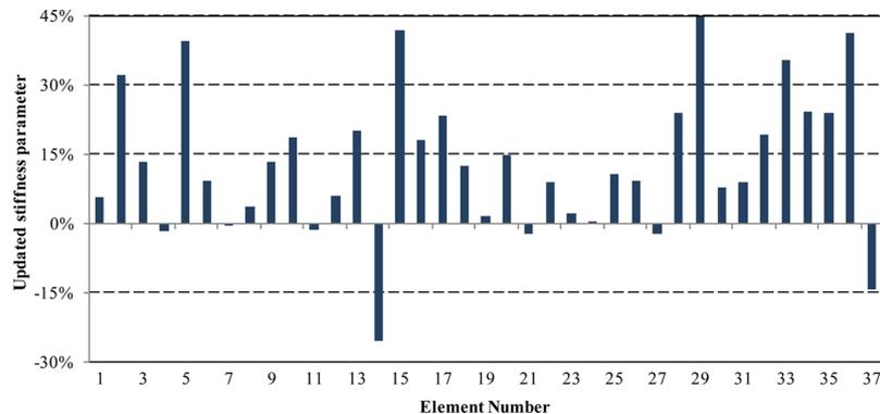
Fig. 4 Updated stiffness parameters of the FE analytical model using first 12 measured frequencies including two torsion modes
