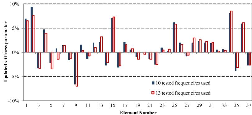
Fig. 6 Updated stiffness parameters of the FE analytical model using 10 and 13 measured frequencies without including two torsion modes
