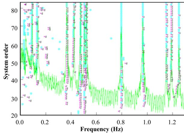
Fig. 2 The stabilisation diagram of measured acceleration data used for the stochastic subspace identification technique
