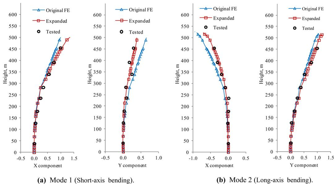
Fig. 4 Expanded first 10 bending modes, compared with the modal readings identified from vibration data and the eigenvectors of the reduced analytical model
