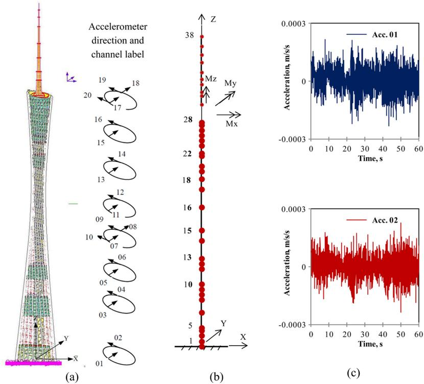
Fig. 1 The Canton Tower benchmark problem: (a) positions of installed accelerometers (after Chen *et al.* 2011), (b) reduced-order finite element model and (c) acceleration measurements of accelerometers 01 and 02
