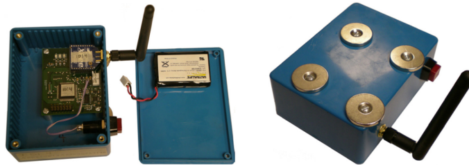
Fig. 1 Sensor node circuit board with enclosure, enclosure lid with Li-Ion battery, and neodymium magnetic mounts
