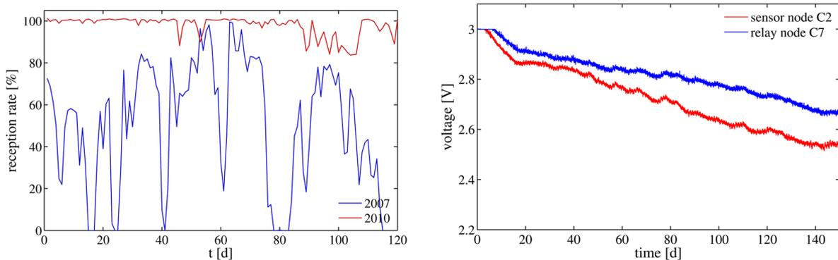
Fig. 10 (a) Delivery ratio of two test periods and (b) supply voltage evolution for nodes C2 and C7
