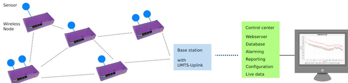
Fig. 4 Overview of the monitoring system architecture
