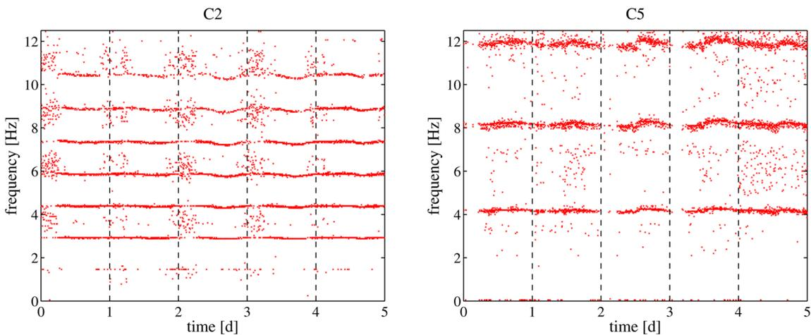
Fig. 9 Natural frequencies of cables C2 and C5
