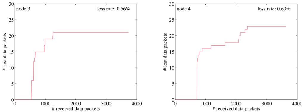
Fig. 7 Data loss of the wireless communications in nodes 3 and 4. The download of the stored data was performed node by node
