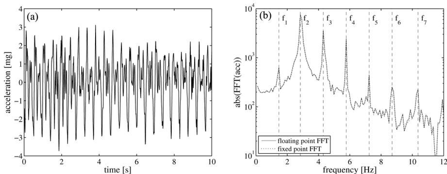
Fig. 2 (a) Ambient vibrations recorded on a stay cable and (b) the spectral amplitude of the integer approximation of FFT compared to the spectral amplitude of the standard floating point FFT
