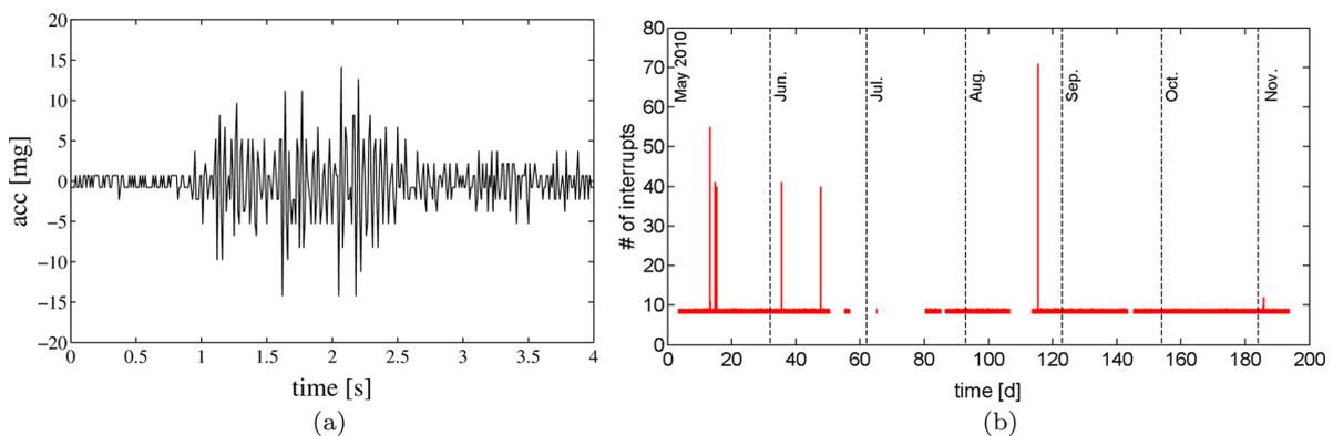
Fig. 13 (1) Time history of accelerations recorded at node 9 and (b) time history of smoke sensors output
