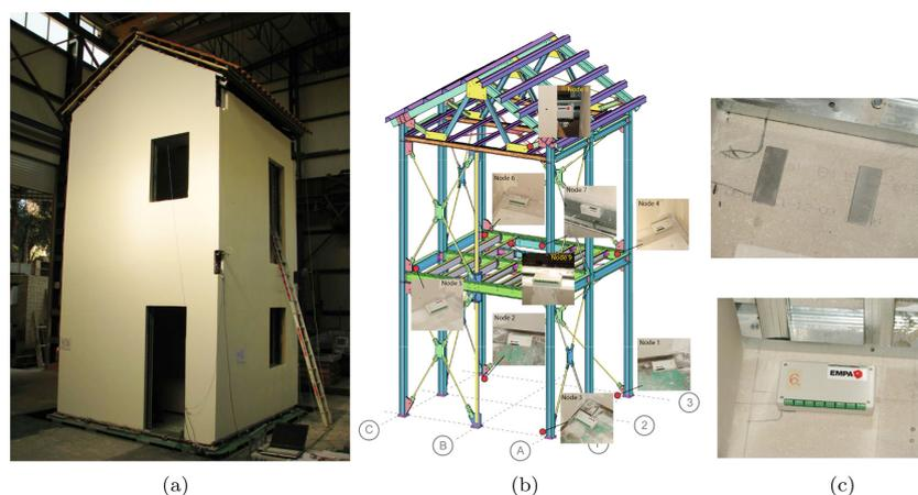
Fig. 5 (a) Mock-up building, (b) location of nodes and (c) sensor node with magnetic footing mounted on the metallic plates
