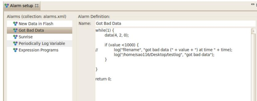
Fig. 12 Alarm setup interface. The left side shows the different alarm setups, while the right side shows the corresponding expressions in xml code
